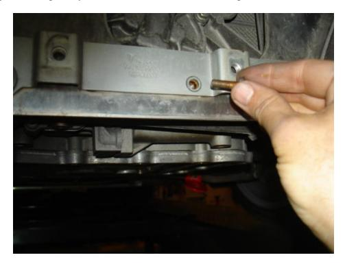
• Tighten the M12 collar nuts on the engine mounts to 63 ftlb.
