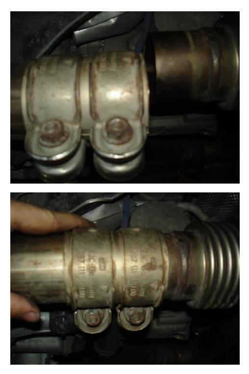
• I placed some Optimoly TA on the threaded studs of the flange joint to the exhaust manifold.
