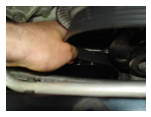
• Then hang it over the alternator pulley (upper left in the pic below).
