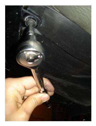
• Next remove the fastening screws on the front-most wheel-well liner. This liner fits under the next piece of wheel-well liner, and so it is necessary to remove the two fastening screws immediately above it.
