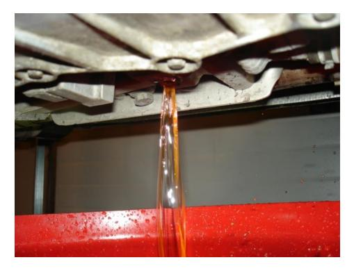
• Once the coolant had drained to a trickle, I then turned to the hose at the inlet side of the water pump. Undo the spring clip on the hose, slide it to the side.
