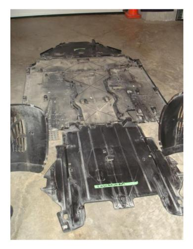
• To remove the belly pans, I start from the rear-most pan. My count of the fastening screws and nuts is based on memory, and so may not be 100% accurate. This pan is held
