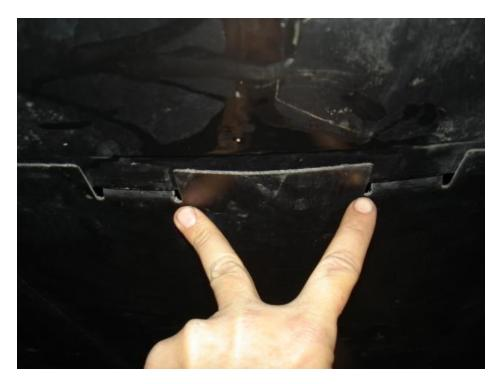
• ...and then install a nut on the third threaded stud from the back on each side of the pan.
