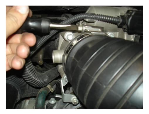
• Route the wire for the electric switch-over valve (3.8L engine) into the omega clip on the right side of the air cleaner housing (sorry for the blurry pic.).
