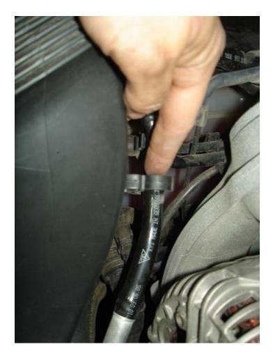
• Gently lift the air cleaner housing out of the fastening lug (pictured below), but not all the way out of the engine compartment because there is one more thing to disconnect.
