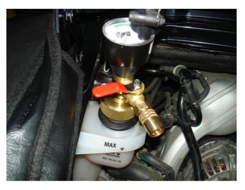
• Then attach the venturi tube to the Airlift. I left the ball valve on the Airlift in the closed position.
