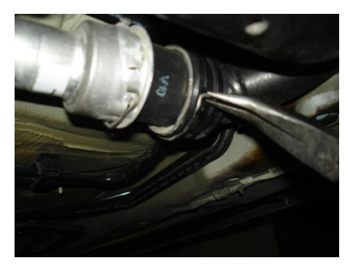
• ... and had to use some force to get the hose out of the coupling, but it did come apart enough to drain the coolant (It required both hands to keep these hoses apart, so I could not get a better picture than the one below).
