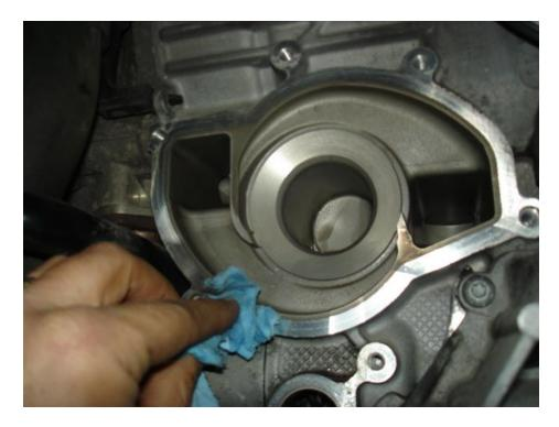
• Apply some degreaser to a clean shop towel to degrease the sealing surface.
