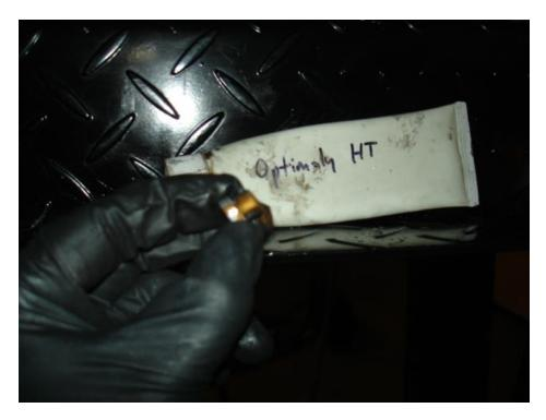
• Torque the drain plug to 7.5 ftlb (90 inch pounds).
