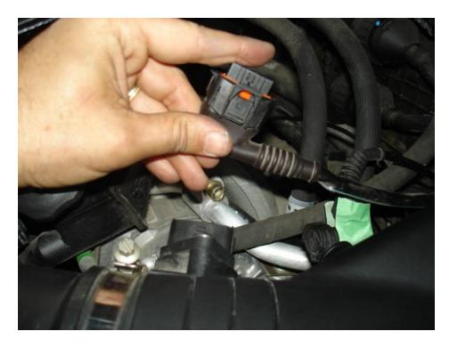
• Next, open the omega clip that holds the MAF meter in place.
