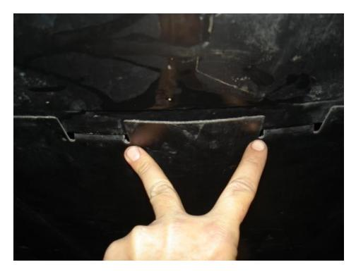
• Finally, the front-most pan is held on by two threaded studs at the back,....
