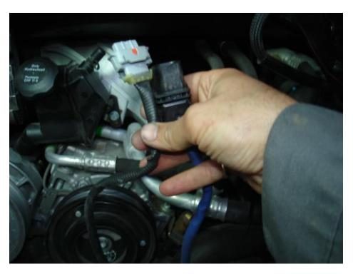
• The pic below shows how the black wire routes aft of the engine carrier and the blue wire routes fore of the engine carrier, and both have clips that hold them in place on the engine carrier.
