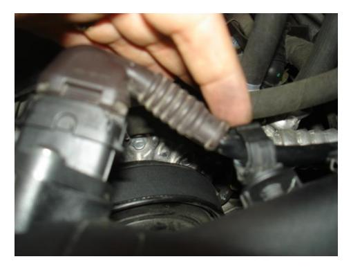
• Place the hose that runs along on the back side of the intake portion of the air cleaner housing into its omega clip.
