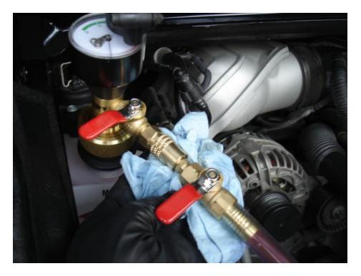
• The resulting fill was at the prefect level. If necessary, top up the coolant level in the expansion reservoir to the appropriate level.
