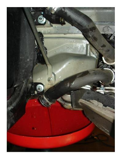
• At the radiators I removed the top hose first, then the bottom hose, then reinstalled the bottom hose followed by the top hose. Ensure all hoses are clean before they are reinstalled. I reinstalled the hoses and then reattached the clips in their original position. In one case, to confirm that I had the clamp properly seated in the coupling on a side of the hose that I could not see, I used an inspection camera.
