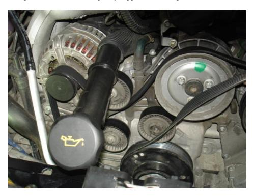
• Next route it under the top idler pulley and over the pulley on the power steering pump, and around the air conditioner compressor pulley.
