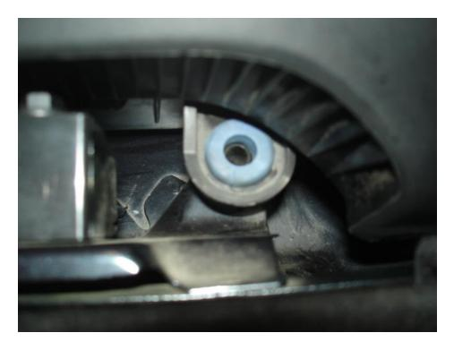
• Once the air cleaner housing is loose, it is possible to access the vacuum line shown below.
