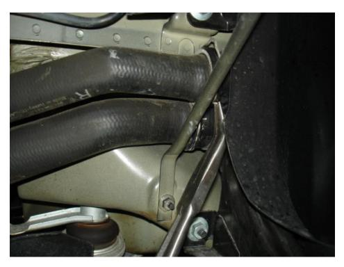
• To do so simply grab the end of the clip on the coupling and lift it so that it is unseated. Do so on both sides of the coupling (in cases where the other side is not accessible, you can grab the clip from another location to unseat and move it. Then the hose can be pulled away from the coolant pipe and drained.
