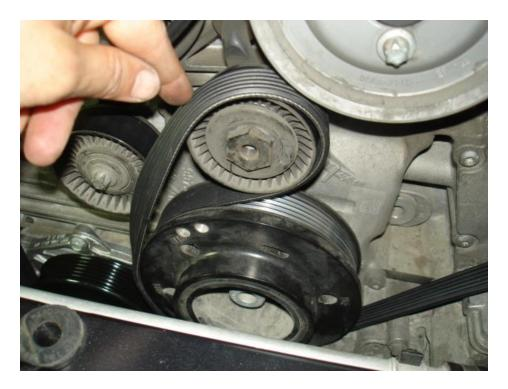
• Place a 24mm wrench/socket on the tensioner bolt, turn the bolt clockwise, slip the belt over the idler pulley beside the tensioner, and then release pressure on the tensioner bolt.
