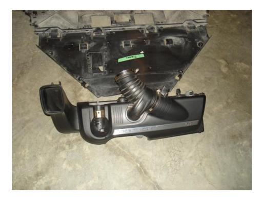
• The air cleaner housing rests in two locating holes in the engine compartment, and there are two rubber grommets (shown below) that sit between the air cleaner housing and the engine compartment. They are loose and usually come out with the air cleaner housing,
