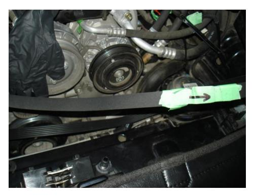
• Fish the belt between the water pump pulley and the engine carrier bracket and place it around the water pump pulley.
