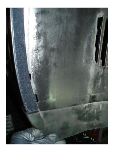
• ...then slid the front-most part of the liner into the front valence and then seated the liner in position under the liner in the top of the wheel well. Replace the fastening screws (remember that the two Torx 27 are for the two screws at the valence).
