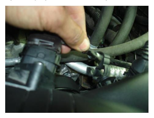
• Next, locate and disconnect the cable from the electric switch-over valve (3.8L engine). Simply press on the wire and lift it off of its flange.
