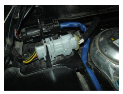
• The wires are held in place with a number of clips. Remove the wires from the clips.
