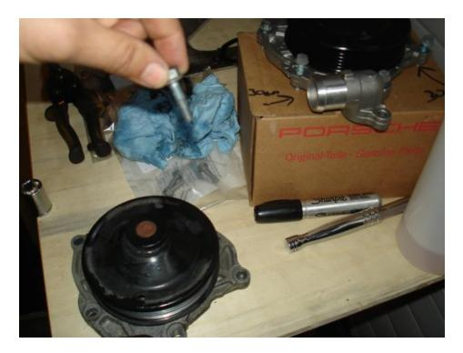
• Clean the sealing surface on the new water pump in the same way that the sealing surface on the crankcase was cleaned.
