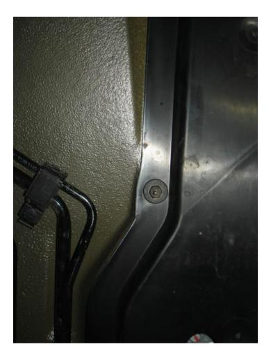
• Next install the side pans. Tuck the pan around the jack point and slide it into the next pan at the front by the jack plate.
