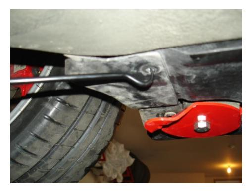
• Next is the 5<sup>th</sup> panel. Line up the flaps at the front of the pan so that the overlap is correct....
