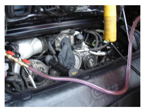
• Ensure the end of the refill hose remains completely submerged during the refill. I added some coolant mix to the pail to ensure there was enough.
