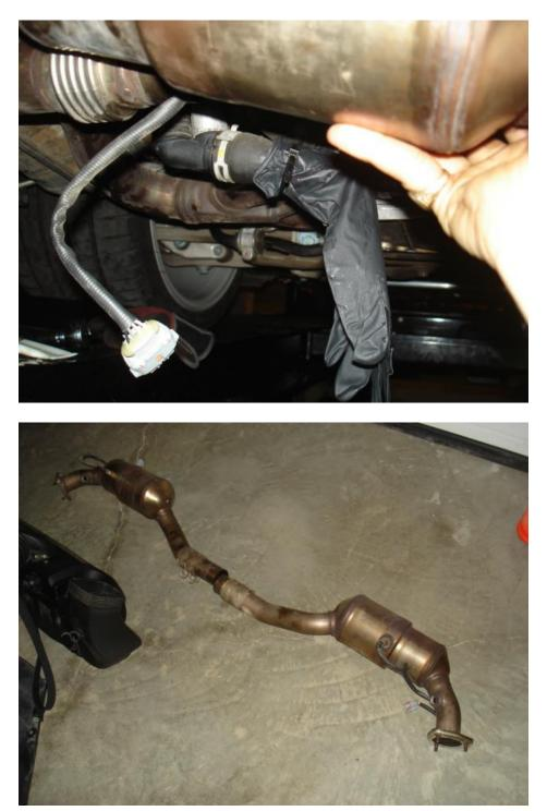
• Next, remove the two bolts (14mm ETorx) that hold the catalytic converter holder to the engine carrier.
