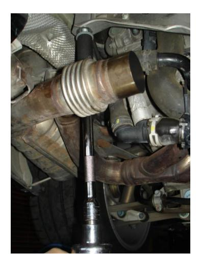
• Then very carefully and slowly lower the engine until the carrier can clear the threaded bolts of the engine mounts. Then remove the engine carrier.
