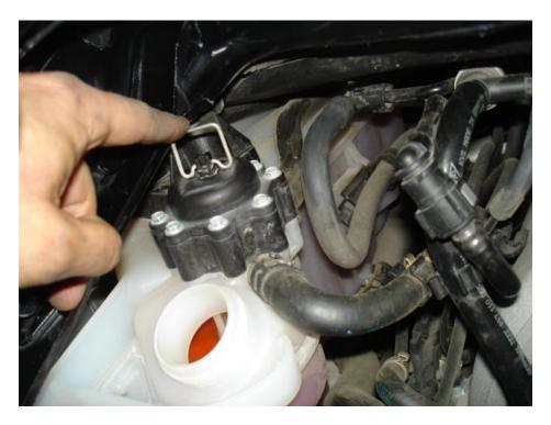
• Locate the coolant drain plug (5mm hex socket) and place a catch container under the plug. Then remove coolant drain plug.
