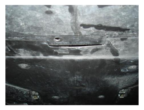
• ...and also fits over 4 studs at the back. Two of the studs are on an angle and it is imperative to release the pan from these studs before pulling the pan away from the one in front of it. It takes some fiddling with pressures in different directions to remove the pan from these angled studs.
