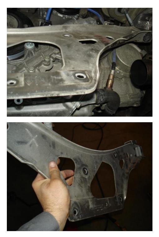
• The pictures below reflect how much the engine is lowered to allow removal of the engine carrier.
