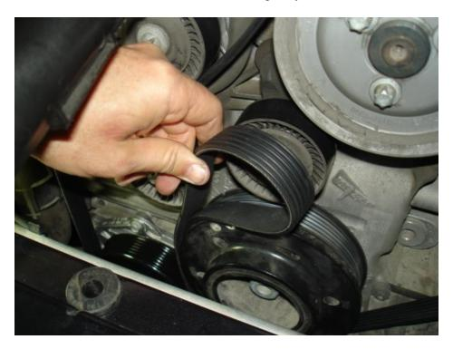
• ...and loop it around the tensioner pulley.
