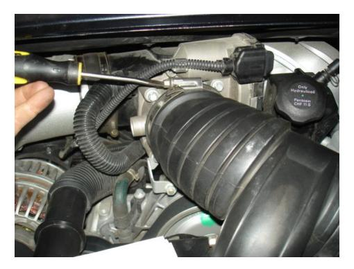
• Then lift the oil filler neck from the air cleaner housing.
