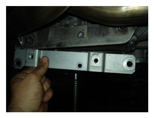
• Next remove the remaining two M10 collar nuts (15 mm) on the engine carrier.
