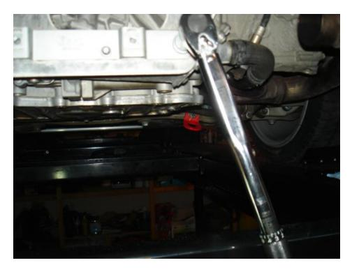
• I put some Optimoly HT on the M6 Torx screw and torqued it to 7.5 ftlb.
