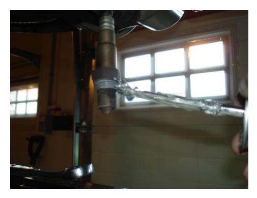
• Tighten the oxygen sensors so they are snug (22mm).
