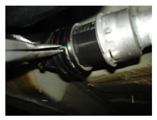
• These were the most difficult ones to disconnect. They are attached to hard lines. On the right side, I removed the plastic bracket that holds the hard line in place...
