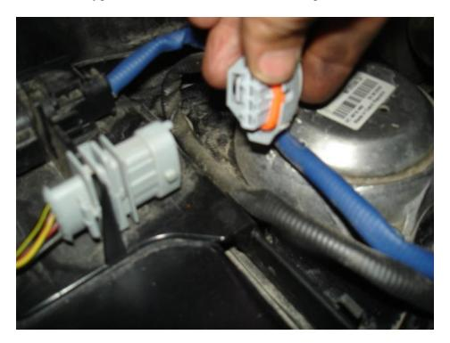
• For the black connector, disconnect it, then remove it from its plastic holder. To do the latter, twist the connector side to side in its holder and it will come out.
