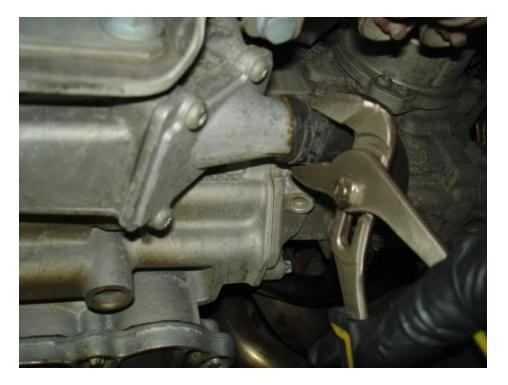
• When the water pump inlet hose had finished draining, to keep any dirt out I placed a latex glove over it and secured the glove with a zip tie.
