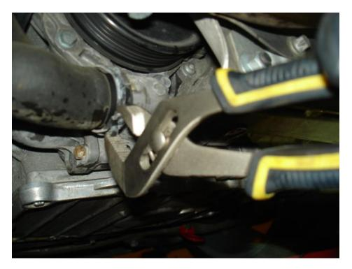
• Place the catch can under the hose, and remove the hose. The hoses held on by spring clips were often somewhat adhered to the pipe on which they seat. To get them off, if
