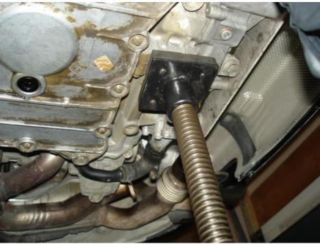
• Then remove the two M10 collar nuts (15mm) and one M6 screw (10mm ETorx) from the engine carrier.
