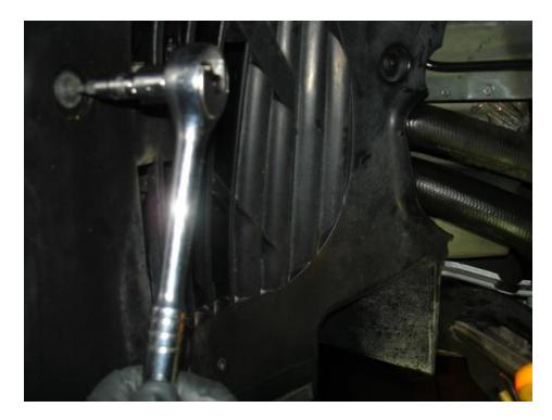
• Then reinstall the wheels, and torque to 96 ftlb.
