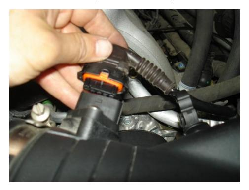
• Place the wire for the MAF into its omega clip.
