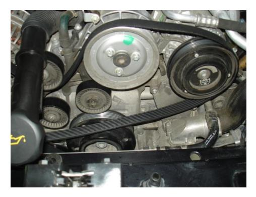
• Then route the belt down around the crankshaft pulley...
