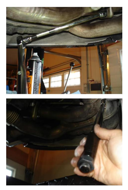
• Then torque the nuts on the clamping sleeve (13mm)
