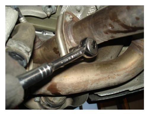
• Note the orientation of the gasket so that it will be replaced correctly. The beading faces the exhaust manifold.
