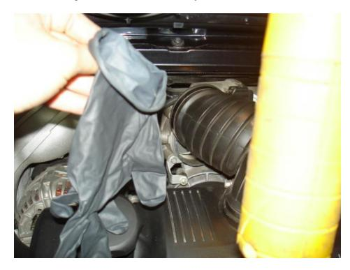
• ...and place the rubber moulding on the throttle body. Tighten the hose clamp on the intake for the MAF.
