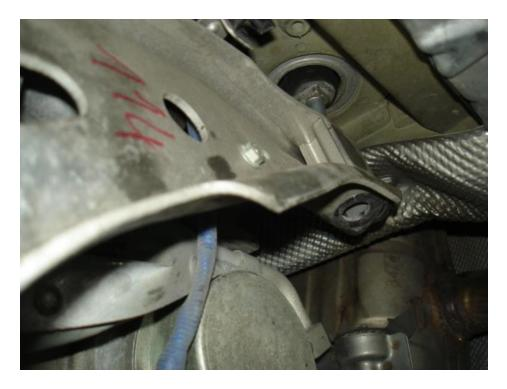
• Place the engine carrier bracket on the threaded mounting studs on the crankcase.
