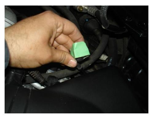
• On the right side of the air cleaner housing is an omega clip holding the wire for the electric switch-over valve. Open the clip and remove the wire (sorry for the blurry pic, but it's the best that my old digital camera that goes through a pair of AAs every two hours would do).
