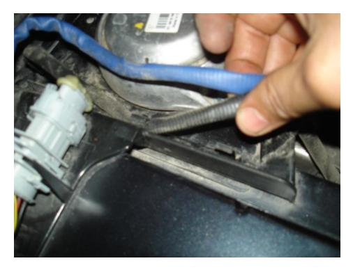
• Disconnect the oxygen sensor connectors from their flanges.
