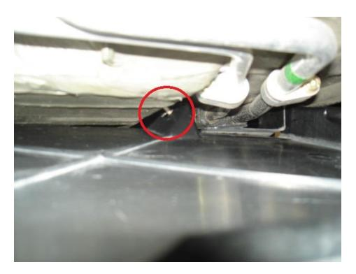
• Next remove the two side pans. These pans are affixed with one fastening screw at the front by the jack plate. Note that these pans slide under the next pan at the front by the jacking plate, as shown below.
