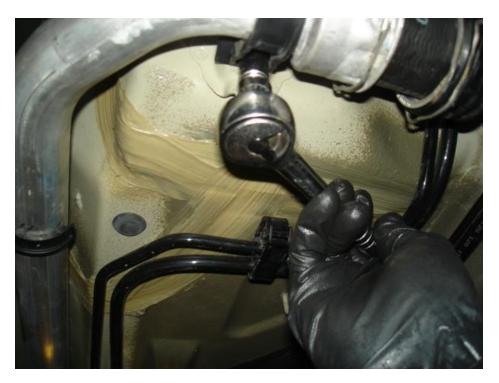
• However, the brackets on the rest of the hard line did not allow the hard line to be moved. It was still necessary to have removed this plastic bracket so that I could twist the hard line down at the Henn coupling. I removed the clip for the Henn coupling...
