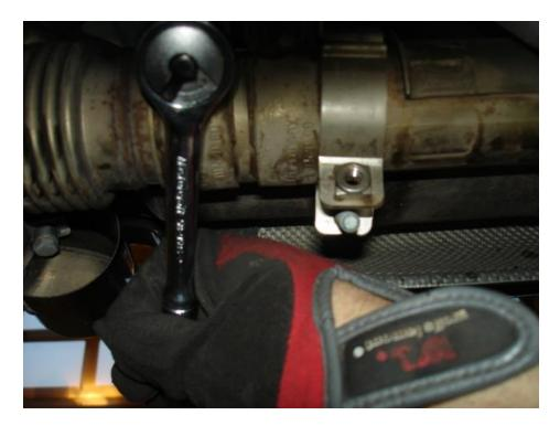
Slide the clamp to the exhaust side.
