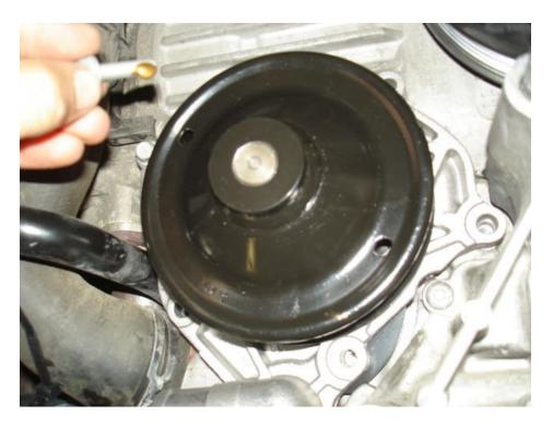
• Tighten all 7 screws in a diagonally opposite sequence (like you would when installing a wheel) to 7.5 ftlb (90 inch pounds).
