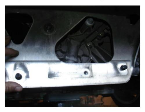
• Next, using your jack raise the engine to the installation position.
