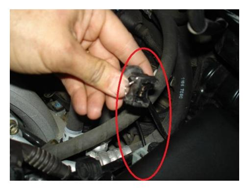
• I cover the ends of these connectors with some painter's tape to keep dust out.
