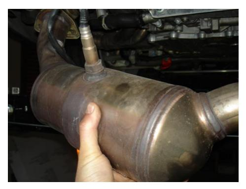
• To install the left side catalytic converter, install the threaded flange end first, then slide the clamping sleeve over the exhaust pipe to hold the catalytic converter in place.
