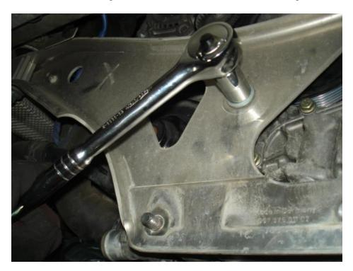
• Using an 18mm deep socket, unscrew the M12 collar nuts on the engine mounts.
