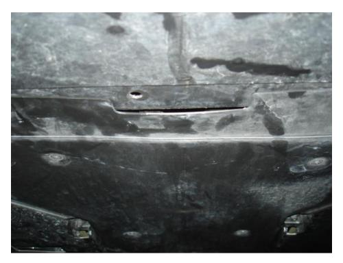
• ...and then lift the back of the pan and place it over the threaded mounting studs paying special attention to getting the pan over the two angled studs.
