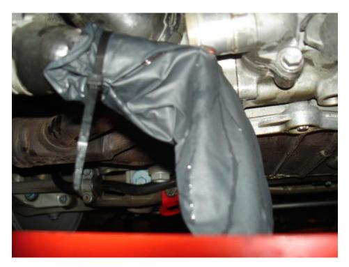
• Once the coolant drain has finished draining, install a new coolant drain plug with new crush washer. I placed some Optimoly HT on the drain plug.
