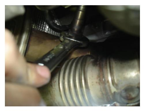
• Now tighten down all of the connections for the catalytic converters. They are all torqued to 17 ftlb. Begin with the lock nuts on the threaded flange joint to the exhaust manifold (10 mm). I had to use a few different length socket extensions to accommodate the end of my torque wrench.
