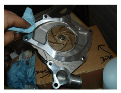
• Next fit the new gasket to the new water pump, and cut the gasket at the 3 connecting points.
