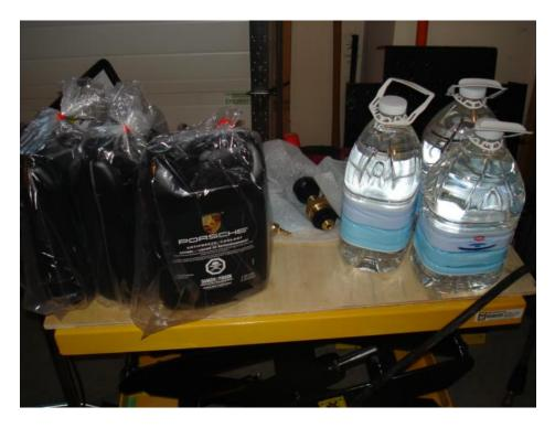
• The coolant comes in 1 gallon jugs (3.78L), and the distilled water comes in 4L containers. To get a 50/50 mix, I first marked the actual level of the coolant in each container.
