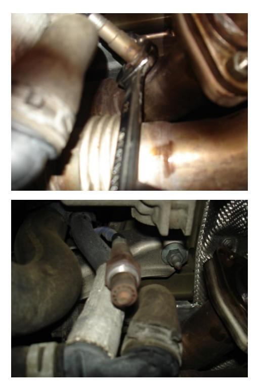
• Next, loosen the two 13mm bolts on the clamping sleeve on the pipe behind the catalytic converter.
