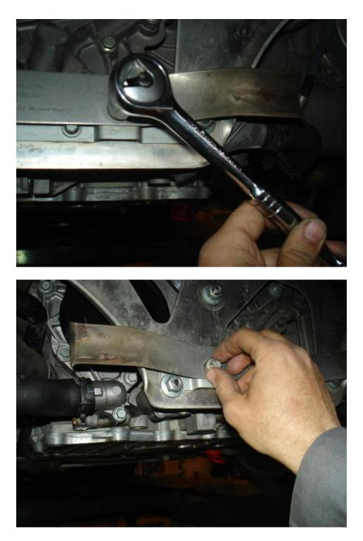
• Remove the catalytic converter holder and set it aside.
