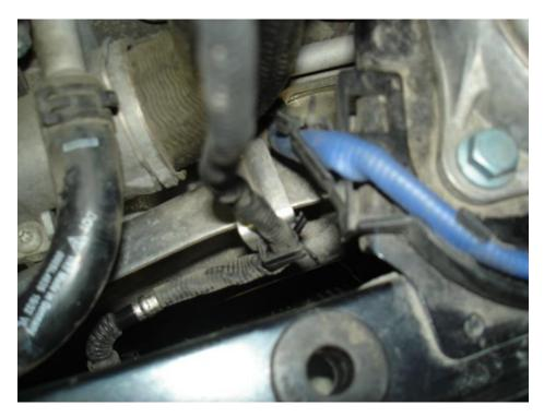
• Next, reconnect the connectors to their flanges and place the black connector back into its plastic holder.
