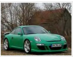
unobtrusive. The spoiler rear hood and the rear wing are made of high-quality Kevlar-Carbon. Aerodynamically optimized RUF side mirrors complete the optical design of the R Kompressor.
