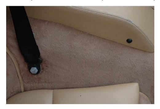
Remove the remaining Phillips screws that hold the frame cover to the frame, and then remove the frame cover.
