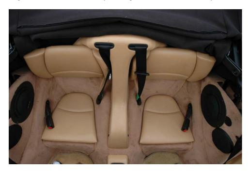
Remove the plastic covers and unbolt the seat belts.
