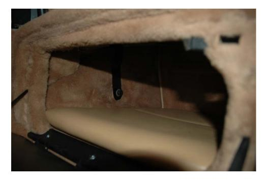
This part of the install was the most difficult for me. The problem was getting the bracket to align at the bottom so the seat belt attaching bolt could be threaded in.
