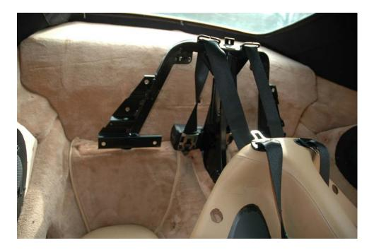
You will also have to unbolt the seat belt retractors and remove them to set the frame cover aside.
