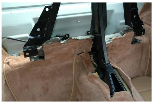
Try to preplan your carpet cuts in advance. I had not made X cuts on the front bolts, so this may have resulted in more carpet cutting than was necessary.
