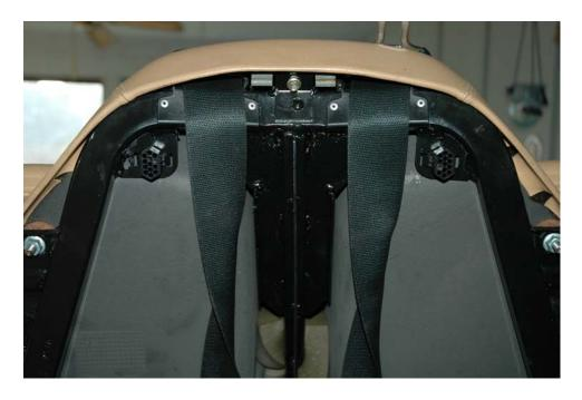
Remove the plastic covers and screws on the very front of the seat assembly
