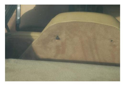
This panel is glued at the bottom so removal will meet with resistance
