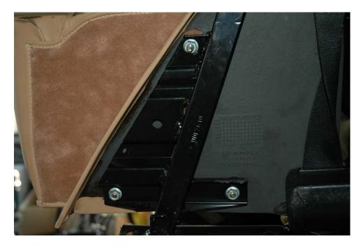
Once the back rests have been removed, remove the small bolt on the backside at the very top of the Rear Seat frame.
