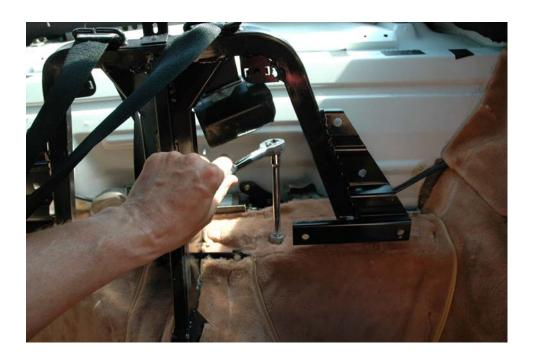
Once all the bolts have been removed, you will need to carefully cut the carpeting and fill padding to remove the Rear Seat frame. In the front section there is a large amount of foam that is attached to the metal frame yoke. Separate this foam from the frame carefully, then remove the frame.
