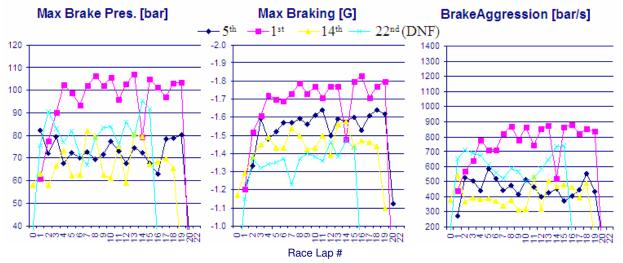
Using the channel report function of i2 is easy to create a table showing the following parameters for each lap. These key performance indicators help you keep tabs of the braking performance of your car and driver package.
