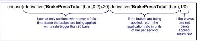
To measure how smoothly a driver releases the brakes we can use the Brake Release Smoothness channel. The Brake Release Smoothness is derived from the difference between a smoothed brake trace and the actual brake trace. This channel is gated so that it only returns values when the driver is releasing the brakes so it doesn't penalize a driver who is aggressive with brake application.
