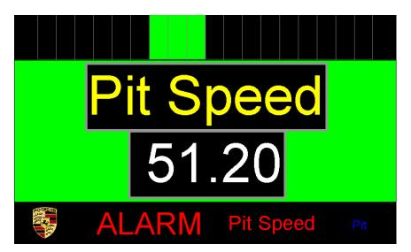
This is red 'over-speed' compared to the target Kph (again in this example the speed is 60 Kph)
