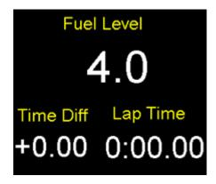
Time Diff is the qualifying mode function to show gain or loss compared to a reference lap.
