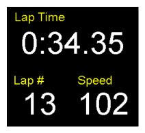
The Lap Time field shows two possible values and is always in the format m:SS.ss
