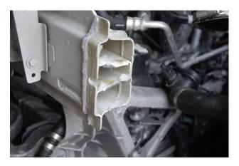
C. It was observed that the welds failed in a brittle manner, exhibited porosity and had insufficient weld build-up. This can be seen (for the left-side weld) in the photo below:
