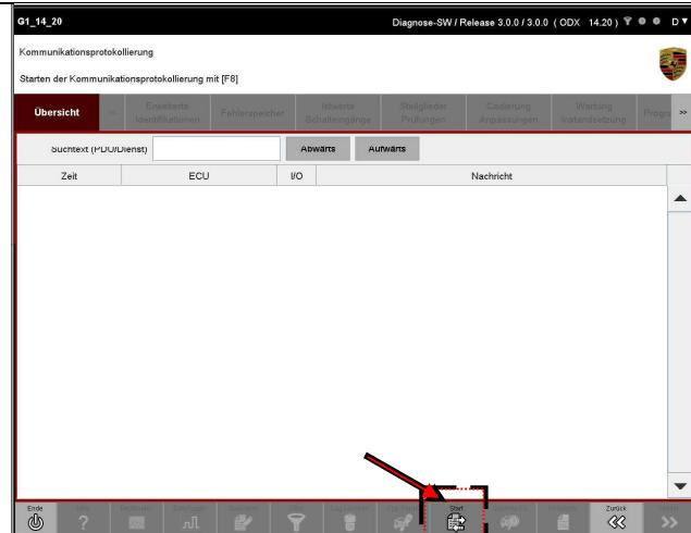
3. The communication between the installed control units and the diagnostic application is now also logged. You can use other functions of the diagnostic application as usual.
