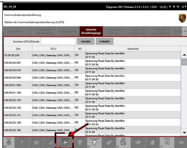
3. A pop-up window appears in which you have to enter the location (A) and the file name (B) under which the communication protocol is to be saved.
