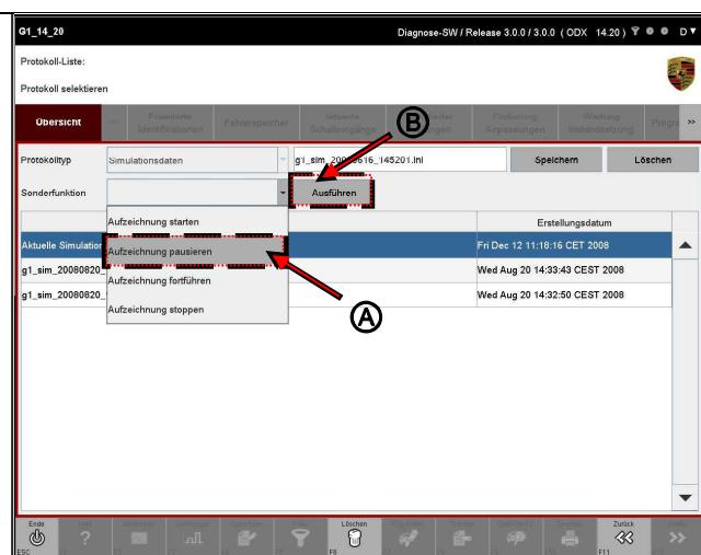
3. To the function Simulation data To exit, press the <F11> key. Now carry out the control unit actions that should not be recorded.
