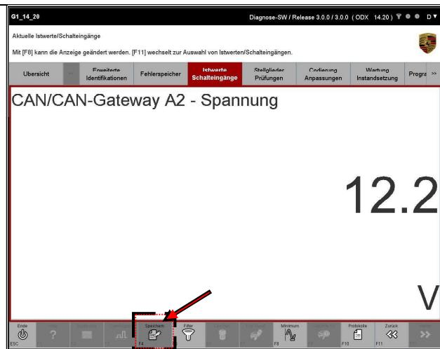
4. If you would like to save information in other screens as well, switch to the corresponding screen and press the <F4> key there again. The information recorded is then included in the same work log. The work log will be expanded to include the new content until it has been finalized / saved.
