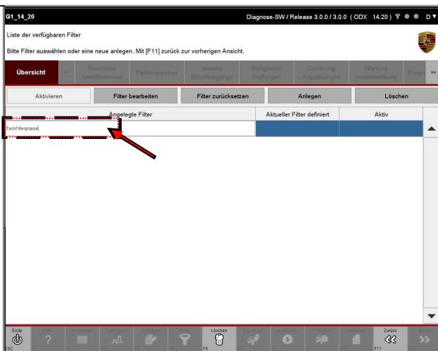
5. To assign the necessary properties to the filter - or to select those elements that should be filtered ?? press the Filter-edit-Button.
