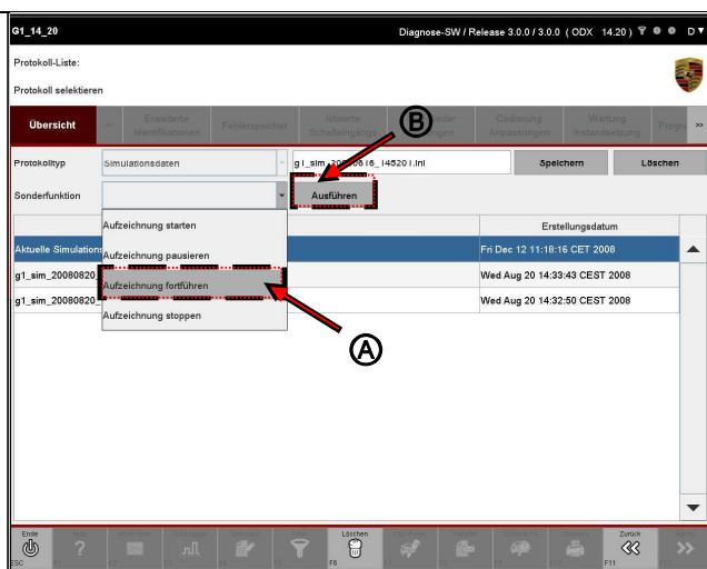
3. From the point at which the recording is continued, the entire diagnostic communication is saved again in the temporary file created previously. All data recorded before the recording was paused is retained. The new data will be appended to the data already recorded.
