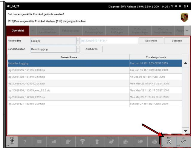
4. If you have confirmed the selection by pressing the <F12> key with YES, the current logging will be deleted. A new logging is then started immediately. The log depth is based on the belowSpecial functions set logging method (basic logging or extended logging).
