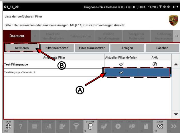
4. In the list of possible filters, the new / changed active filter is indicated by the icon in the split active displayed.
