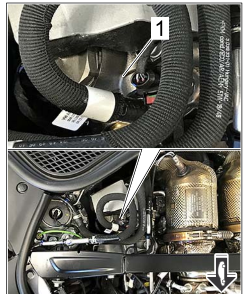
Contact point on high-pressure pump
