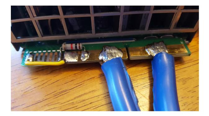
Upon plugging in the power supply, you should see the green light come on. If the light turns orange, the internal voltage is set above over-voltage protection. Since we need around 14v anyway, we will be disabling OVP. Simply solder a bridge between the pictured components.
