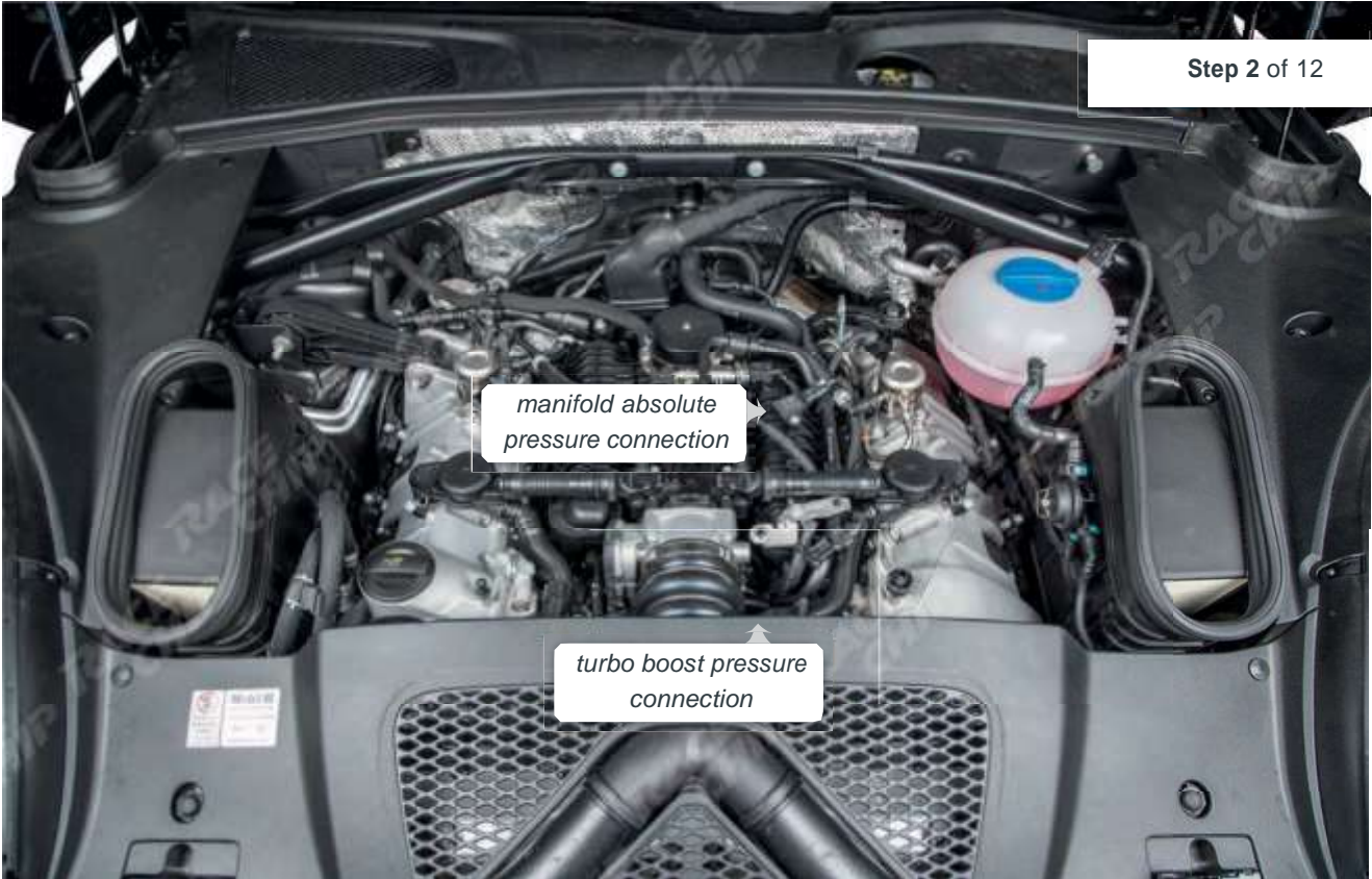
This image shows the connections that are relevant for the installation in your vehicle.
