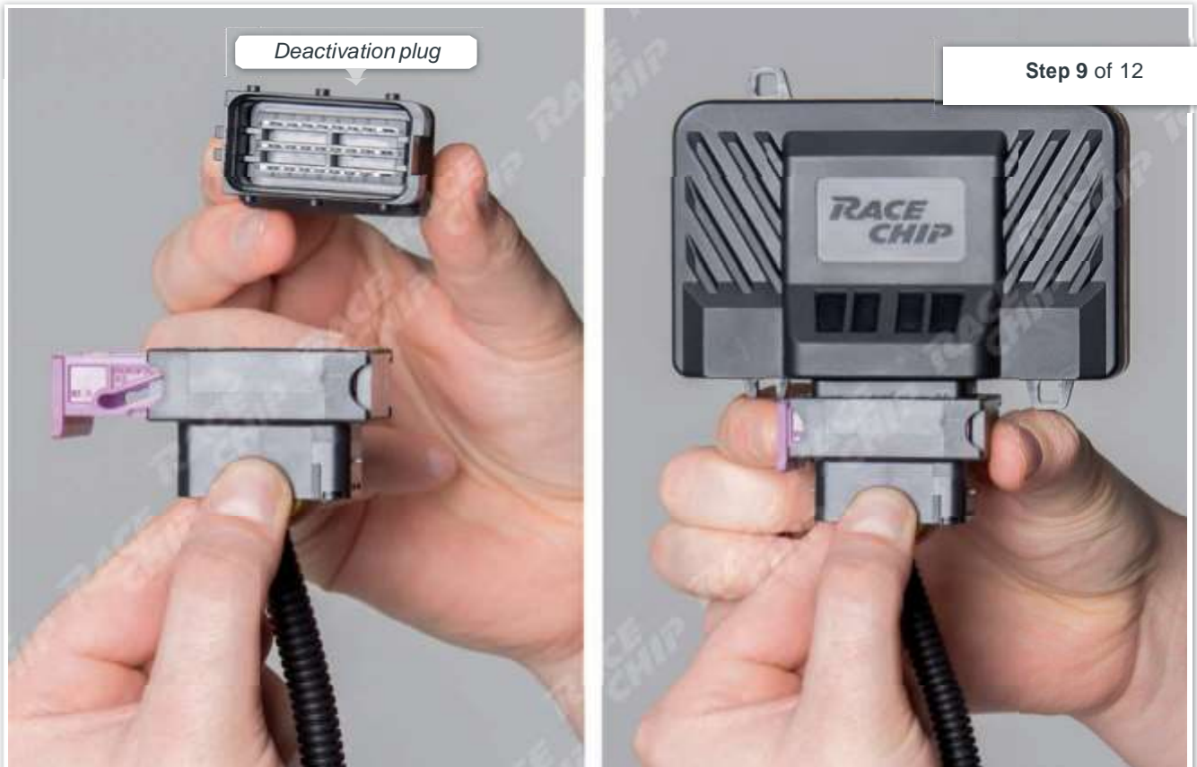
Wiring harness with deactivation plug removed
