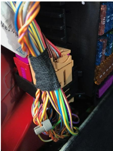
981 shown here. 996 GT3/997 GT3 and 987.1 use White AiM CAN+ to blue, Blue AIM CAN- to grey
