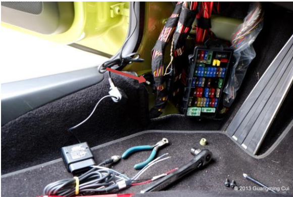
Above: Carpet cover off. Arrow pointing to ground stud. CAN twisted pair in largest bundle towards rear of car. Cut and peel back canvas tape. For 996 GT3 and 997 GT3, unwind blue and grey twisted pair 1.5"-2.5" to separate wires. You will HAVE to dig inside the thick bundle of wires to find the blue/grey twisted pair of wires on the 996 GT3.
