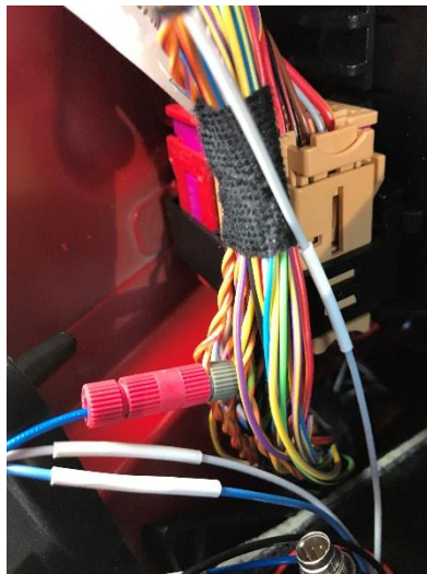
981 shown here. 996 GT3/997 GT3 and 987.1 use White AiM CAN+ to blue, Blue AIM CAN- to grey
