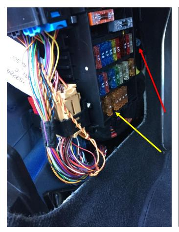
Extract the twisted pair from the bundle. CAREFULLY use an Exacto knife or sharp scissors to cut the black fabric tape binding the loom below the connectors.
