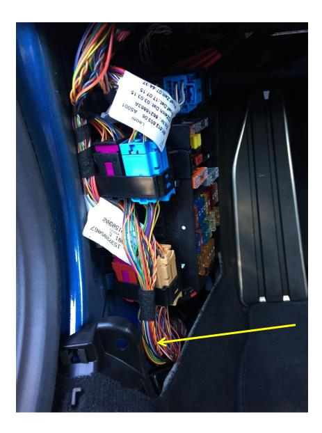
With the panel off, here are the two "gateway" connectors that connect the rear harness to the dash and instrument cluster harnesses.
