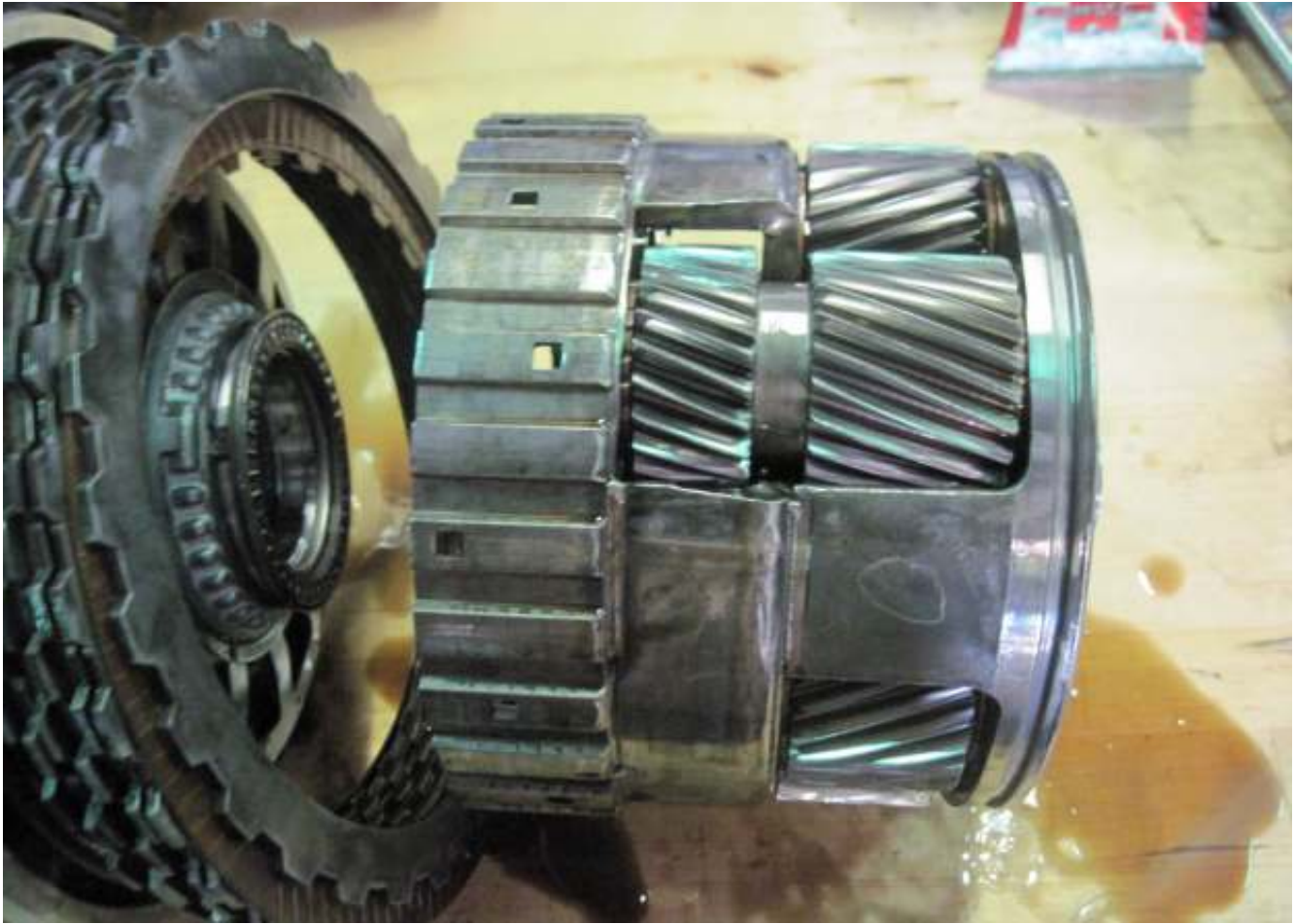
Ravigneaux planetary gear set and D brake frictions and steels
