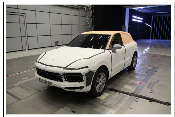
Figure 4. Full-scale wind tunnel model ('Aerobuck').
