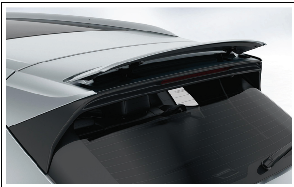
Figure 28. Adaptive roof spoiler of the Turbo.
