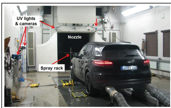
Figure 35. Soiling test setup in the FKFS thermal wind tunnel.
