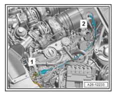
Remove, disconnect and free up the connector from the bracket.
