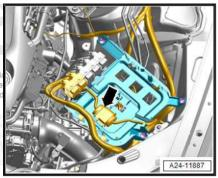
Equipment version with particulate filter: remove the connector -1- for the Exhaust Gas Temperature Sensor 3 Bank 2 -G497- from the bracket, disconnect it and free up the wire.
