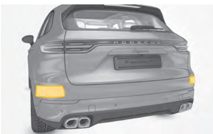
Fig. 87: Radar sensors in rear bumper
