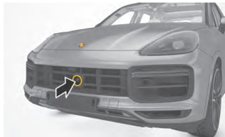
Fig. 2: Radar sensor position
