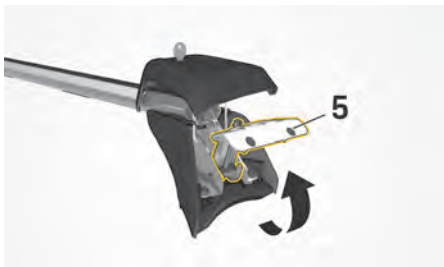
Fig. 177: Swivel the fastening bracket upward and engage it in the carrier support
