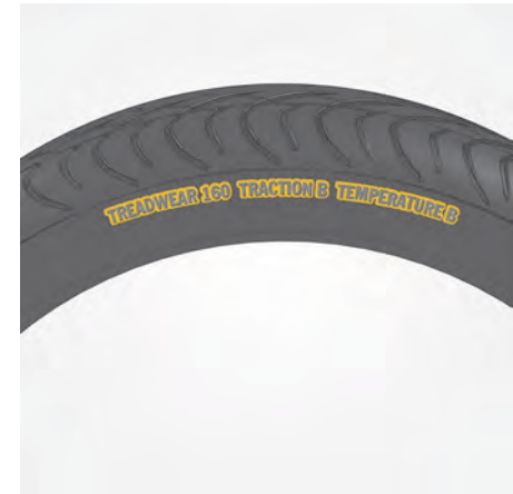
Fig. 238: Treadwear, Traction and Temperature of the Tire Quality grades can be found where applicable on the tire sidewall between tread shoulder and maximum section width. All passenger vehicle tires must conform to Federal Safety Requirements in addition to these grades. Quality grades can be found where applicable.
