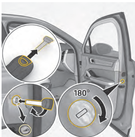
Fig. 40: Performing emergency locking of the passenger's door
