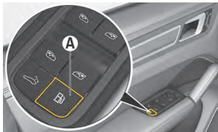
Fig. 160: Button A: Starting fuel tank ventilation and re-leasing filler flap (E-Hybrid vehicles)
