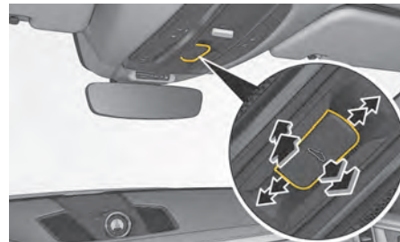
Fig. 166: Opening and closing the roof system
