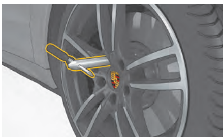
Fig. 244: Screw in one assembly aid on vehicles without PCCB
