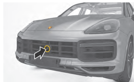
Fig. 9: Radar sensor position
