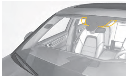
Fig. 126: Attaching toll devices
