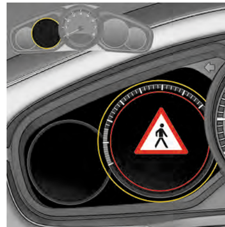
Fig. 128: Pedestrian warning on instrument cluster
