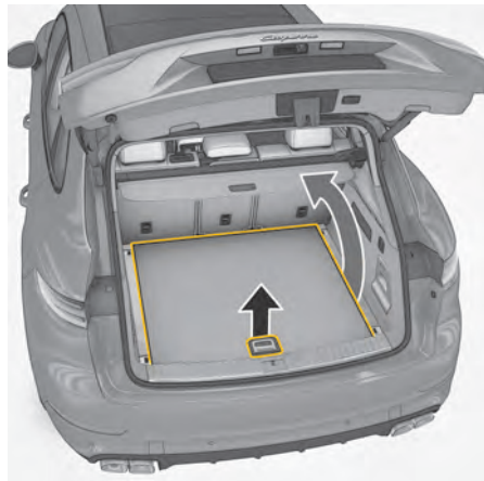
Fig. 101: Opening the cargo area floor
