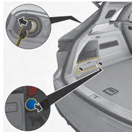
Fig. 49: Performing emergency release of the vehicle plug (vehicles with DVD changer)
