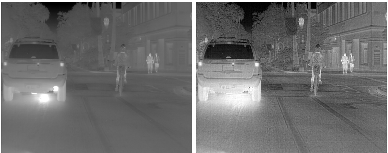
Figure 11: Example of a difficult scene to handle for an IR-sensor. To the left: The hot exhaust pipe stretch out the dynamic range and make it difficult to see fine details with a normal image adjustment algorithm. To the right: The same image with STACE algorithm applied.
