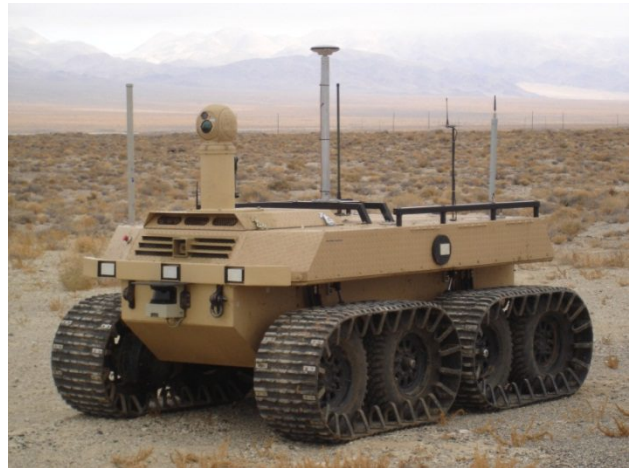
Figure 5: A gimbaled ISR sensor installed on an Unmanned Ground Vehicle, providing the remote human controller or computer driver with excellent intelligence, surveillance and reconnaissance ability.
