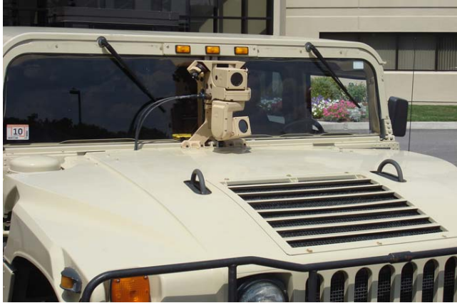
Figure 1: A militarized DVE (Drivers Vision Enhancement) system installed on a Humvee, providing unprecedented night vision driving with awareness far beyond what headlights can provide.
