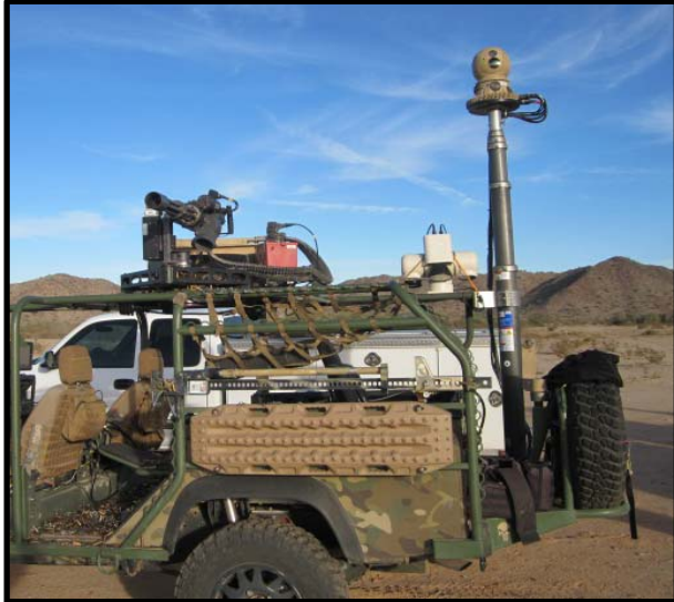
Figure 6: A gimbaled ISR sensor installed on a retractable post on a Land Rover.
