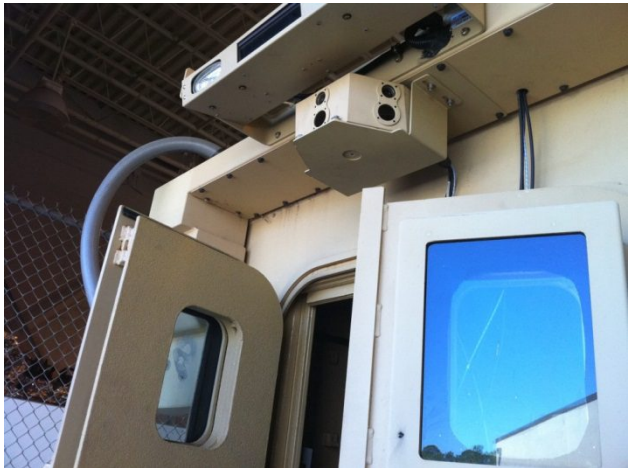
Figure 3: FLIR's Wide Eye sensor provides 180 Degree field of view for situation awareness and force protection.
