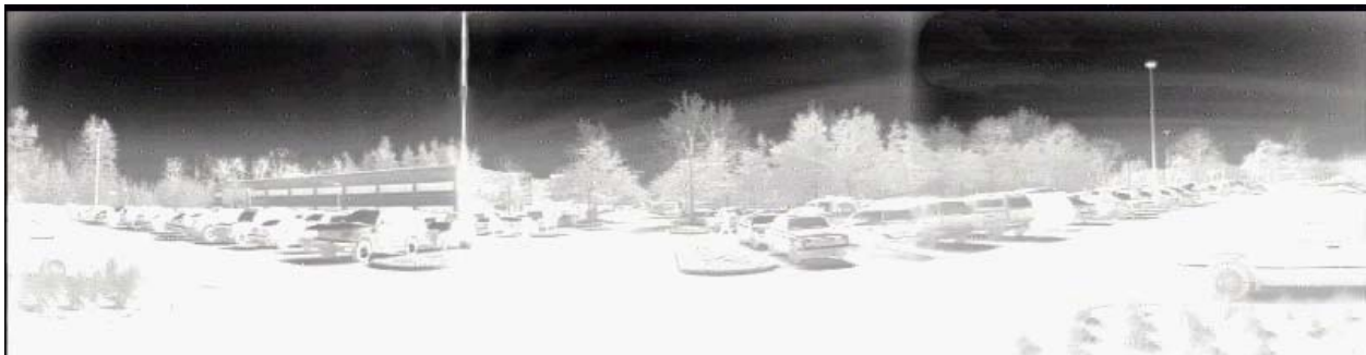
Figure 4: 180 degree wide stitched image from three infrared sensors mounted on a vehicle.
