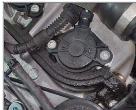
Sample illustration: Oil leak in the camshaft phaser
