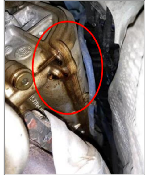
Sample illustration: Oil leak on cylinder head cover
