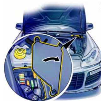
Fuse box in engine compartment
