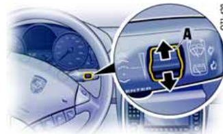
Rain sensor rotary switch
