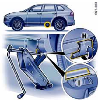
Vehicles with side member panels Rear jacking point
