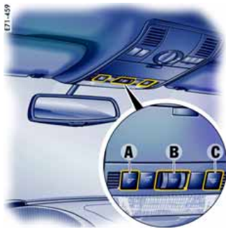
A, C - Switch for individual reading lights B - Switch for interior light
