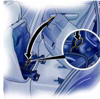
7. Insert mounting hook on the seat cushion in the eyelet of the backrest ( arrow ).
