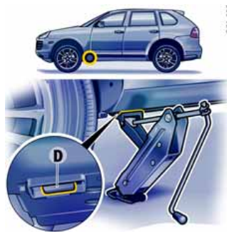
Vehicles with running board Front jacking point
