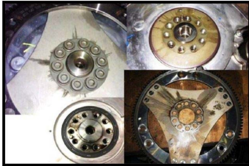
Oil leak on flywheel/drive plate
