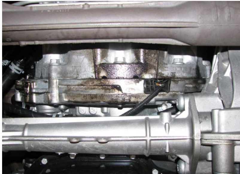
Example of oil leaks on the engine
