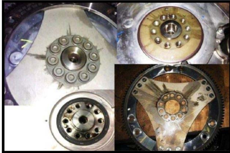
Oil leak via the crankshaft/flywheel sealing ring
