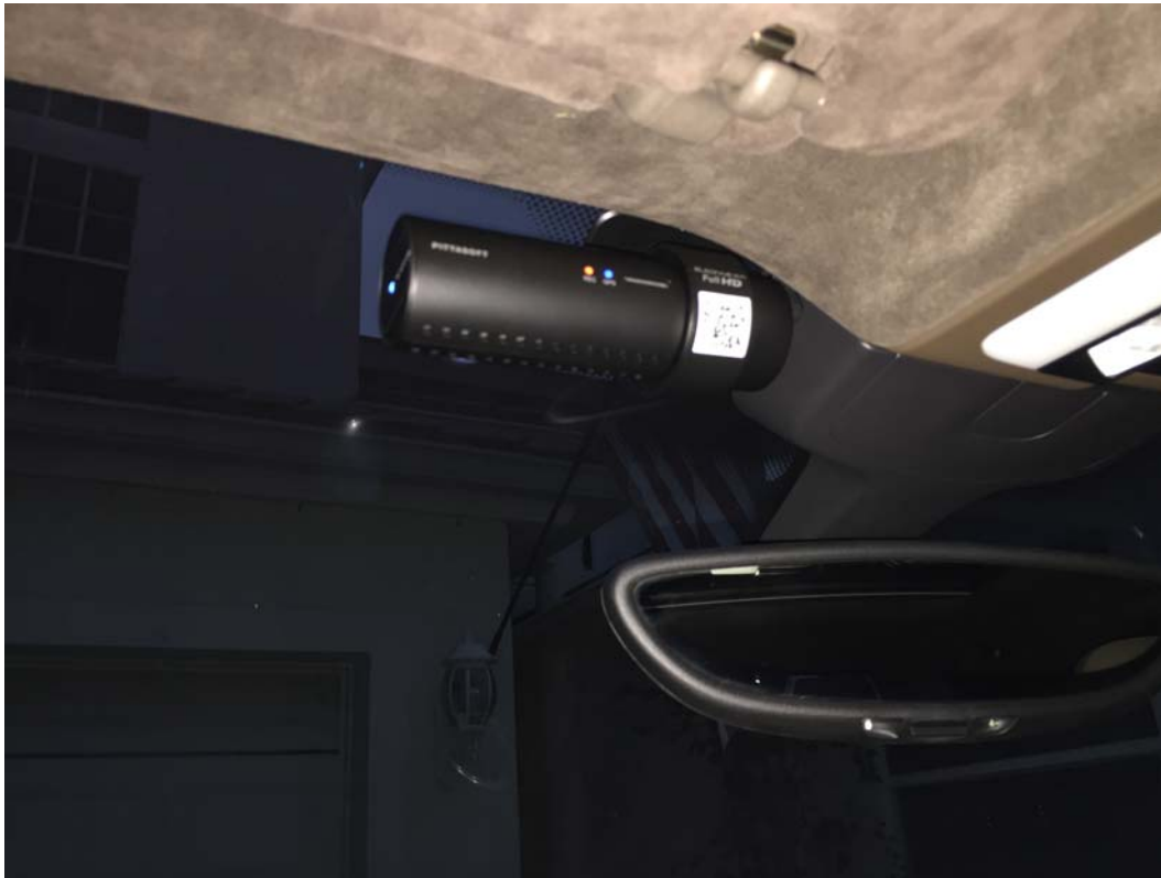
Finished Front Camera installation (below)
