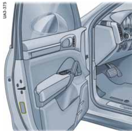
Safety compliance sticker
