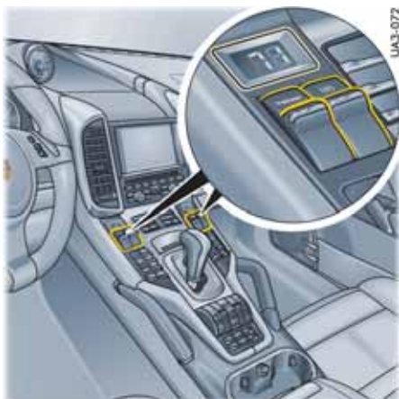
Temperature and air quantity, front control panel
