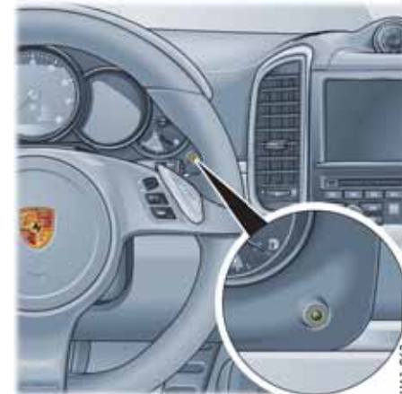
Interior temperature sensor
