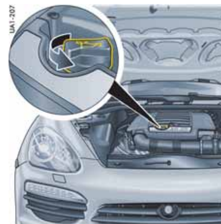
Engine oil filling point on V6 engine
