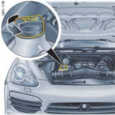
Engine oil filling point on V8 engine
