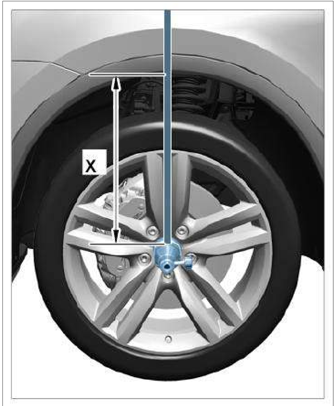
Fig 1: Identifying Front Axle Height
