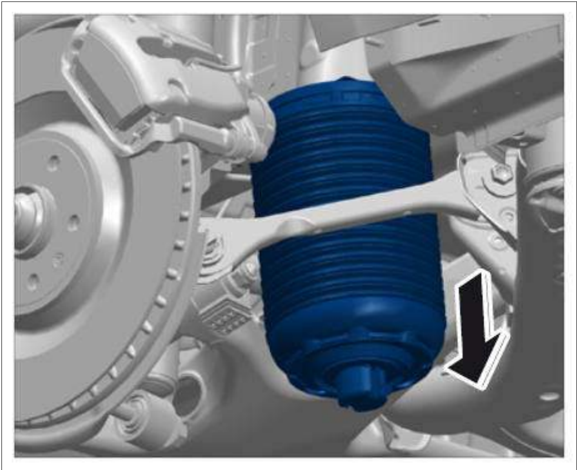
Fig 5: Removing Air Spring
