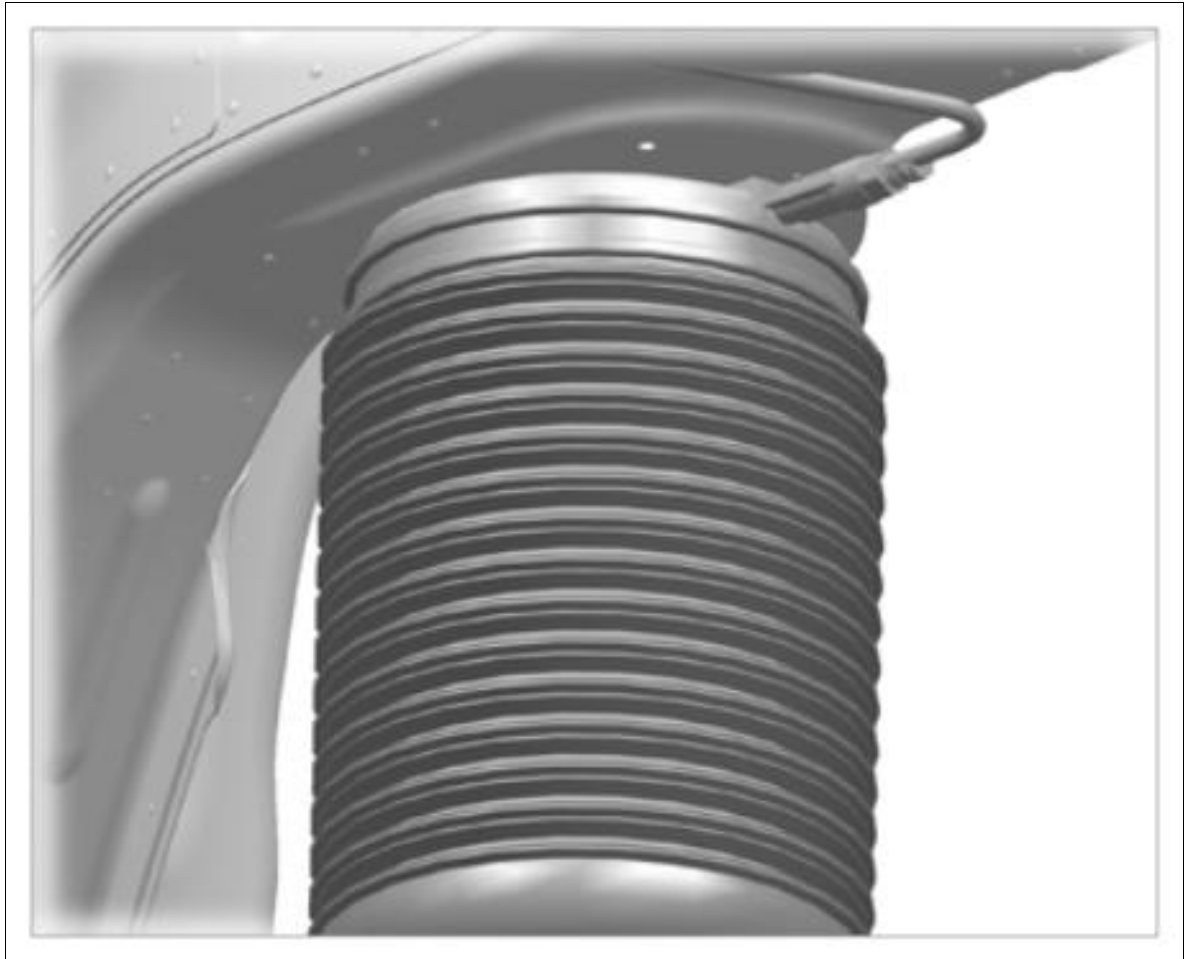
Fig 1: Identifying Air Spring Rolling Creases
