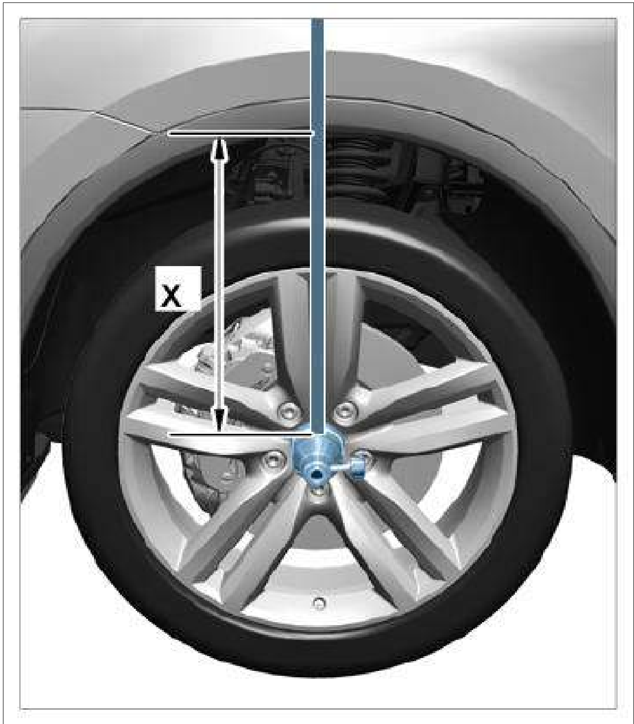
Fig 1: Identifying Rear Axle Point Height
