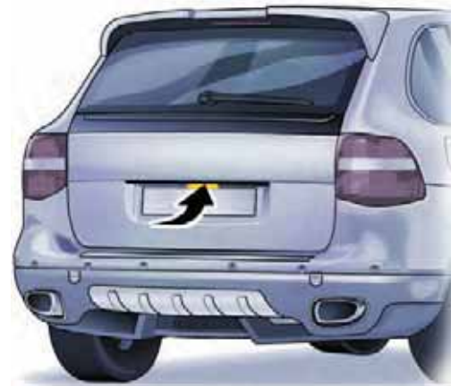
Option 1 – Press the release button on the rear lid.
