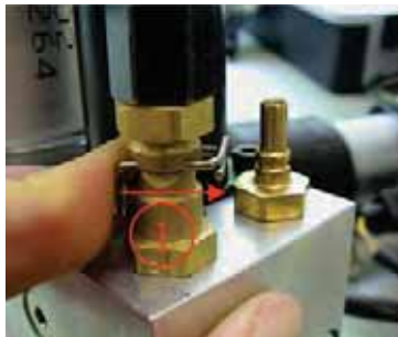
Removing the quick connectors.
