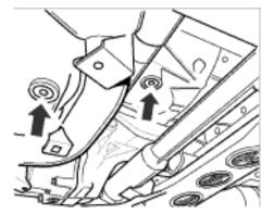
4. Clean oil drain plugs and screw in with new aluminium sealing ring. Tightening torque 50 Nm (37 ftlb.).
