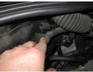
• Using a flathead screwdriver, gently pry up the **two** connectors holding the wire harness to the rear of the right-hand engine compartment side panel.
