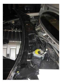
• Depress the far side of the connector (as shown in the pic below) to separate the connector, then set the cowl aside.
