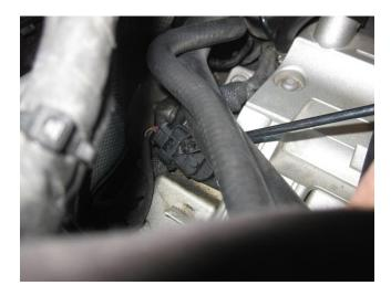
• Next release and pull off the vacuum hose. I had some difficulty with this connector. Pressing in on both sides would not produce enough diameter to release it. What worked for me was to use my flathead screwdriver to release both sides of the connector.
