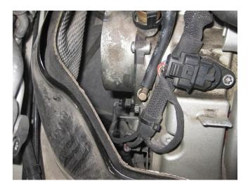
• To get a little more clearance, remove the wiring clip from the camshaft position sensor. Lifting on the tab with a flathead screwdriver releases it.
