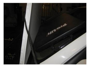
• Then, use a flathead screwdriver to disengage the clip that holds the shock to the hood.
