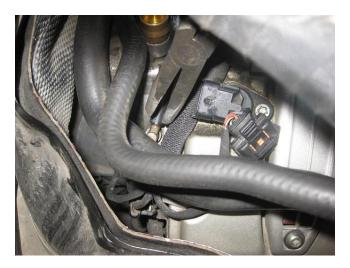
• If you removed the grommet from the flange with the vacuum line, reinstall it and then reinstall that vacuum line on the top of the vacuum pump.
