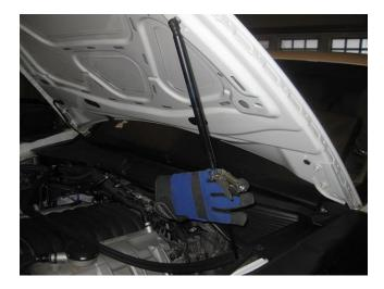
• Close the hood. To ensure the flange of the cowl is fully seated, run the rubber hammer across the full length of the channel.
