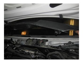
• The pictures below show the cowl flipped over so the connector can be seen.
