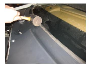
• When you get to the end, use the handle of a screwdriver where the rubber hammer won't fit.
