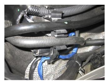
• Reinstall the wiring harness to the right-hand engine compartment side cover by pressing the clips over the threaded screws on the panel.
