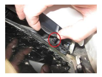
• Then, ensuring that the tangs on the right side are safely placed, as described above for removal of the cowl, gently press the cowl toward the right side causing it to flex up toward the hood and when there is sufficient clearance GENTLY fish the cowl around the left hood hinge (note that you also have to, at the same time, ensure the opening for the left windshield wiper arm is clearing the bolt for said wiper arm).
