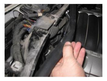
• Open the clamp on the smaller wire harness under the cowl and release the wire.
