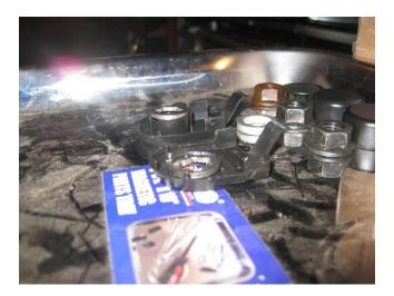
• Next put a puller on the left side wiper arm. There is not a plastic base on this one. I had to adjust my puller as shown below (in an L rather than an H configuration) to get it to fit.
