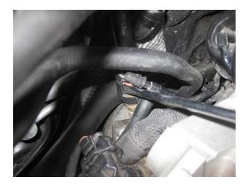
• Gently move the vacuum line toward the front of the car, out of the way. This line goes through a grommet on the flange on which the right-hand engine compartment side panel sits, so it can be released from that flange to move it more out of the way. Below is a pic of the line with its rubber grommet sitting in the flange.
