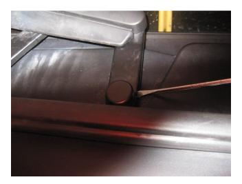
• Unscrew the nuts. Note that the nut on the right side (throughout this document the Porsche convention of left--NA driver's side--and right--NA passenger's side--is used) has an aluminum washer that comes off. Also note that there are hexagonal washers under the arms in the plastic holders (to be shown later).
