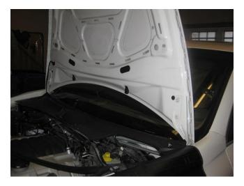
• The flange does not easily stay seated in the channel. To help with putting pressure on the flange, at this point I installed the 2 screws in the right side and installed the panel that sits on the left side of the cowl.
