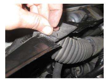
• When doing so, ensure that the grommet is properly fitted into the flanges on both sides.
