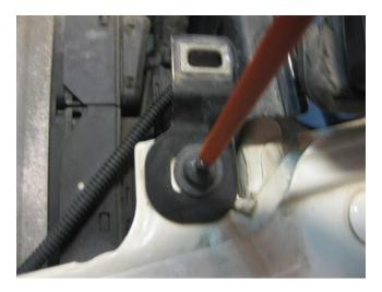
• The third screw is under the main wire harness, as shown below.
