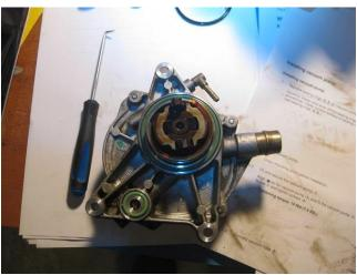
• Prior to installing the vacuum pump, clean the area on the head with a clean, lint free shop towel.
