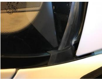
• Reinstall the engine compartment seal. Make sure to go around the whole perimeter of the seal to ensure that it is seated correctly.
