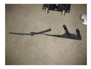
• Note for reassembly that the right-most plastic base for this wiper arm is thicker than the left one (recall that I'm using the Porsche convention for R and L).
