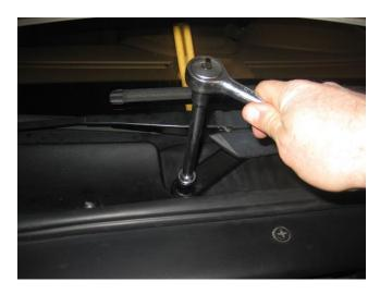
• Put something protective around the hood shock and clamp it to hold it in the extended position (I used a glove)
