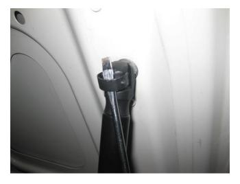
While holding the hood in one hand, with the other hand remove the shock from the ball
