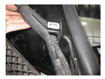
• Reinstall the small wiring harness in its clip on the centre engine compartment shield and reinstall the main wiring harness in its clip on the same shield (I didn't get a pic of the latter but you can't miss it).
