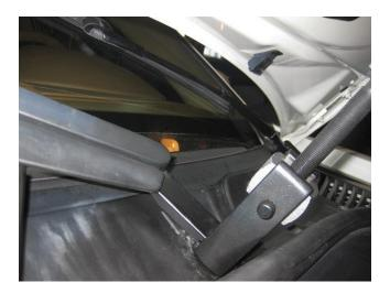
• ...and then to use a different puller with a thinner bolt to get it the rest of the way (this puller's arms had hooks on the pulling arms that were too curved to fit for the initial pull).
