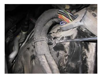
• Gently lift the main electric wire harness with its rubber seal out of its installation position. It will move just far enough to allow the removal of the right-hand engine compartment side panel.
