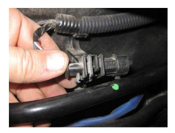
• The bottom one has a small hook on the connector holding it in the clip. So, gently twist it up and away from the right-hand engine compartment side panel and it will then slide out of the clip.
