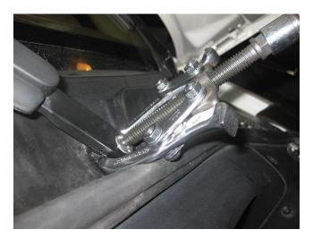
• With the right wiper arm free at both locating points, it can then be removed.
