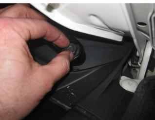
• Place the each plastic base over its respective wiper bolt for the right side wiper arm and put the arm in position.
