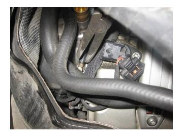
• For more clearance, remove the smaller wiring harness from the centre panel of the engine compartment by sliding its rubber grommet out and setting it aside on the cowl.
