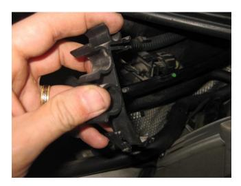
• Gently remove the wires from the clip on the bottom (circled in red).
