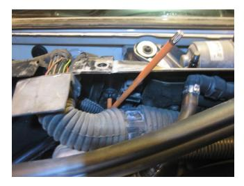
• Now gently lift the right-hand engine compartment side panel, being careful not to snag it on any wires/hoses/lines.
