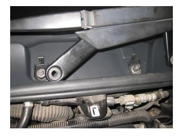
• Put the washer in the right-most position, then start both nuts for this wiper arm.
