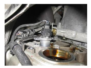
• The solenoid has an o-ring, so ensure that the old o-ring comes out with the solenoid. If it didn't, use a mirror and a light to find and remove it. The o-ring is shown in the (blurry) pic below (circled in red).
