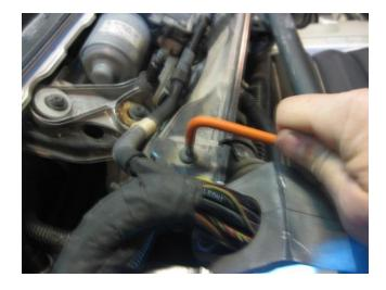
• Note that the screw on the fender has a washer.
