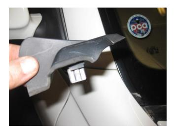
• Loosen the four screws on the cowl (these do not come out completely so just loosen them).
