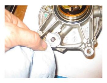
• Apply some motor oil to the new o-rings and install them in the vacuum pump.
