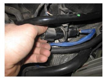
• Slide the top connector from the clip on the right-hand engine compartment side panel. This one slides easily off of the clip.
