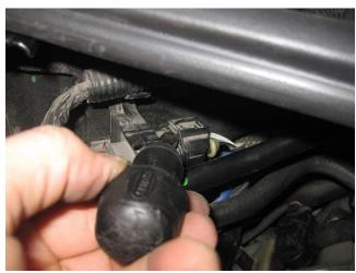
• Unclip the lower connector as shown below (press on the release).
