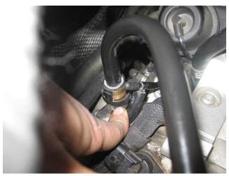
• Next, reinstall the electrical connector on the camshaft position sensor.
