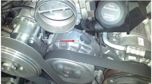
I masked off the carbon fiber heat shield on both sides - hole drilling location on front and entire back - so I could use a hole saw to create the space for the intake pipe without scratching or having the hole cutout be rough around the edges.
