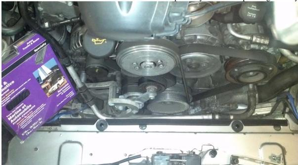
I drilled this hole in the housing so I could mount the standoff & support bracket to something solid. I covered the intake and other engine parts with rags when drilling, then vacuumed up the shaving to make
