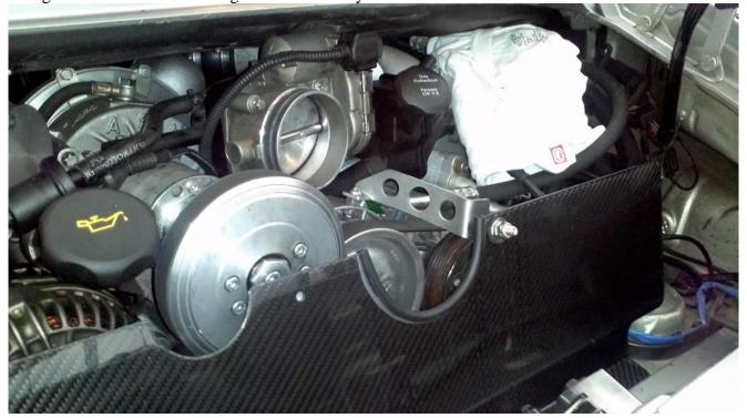
...and there you have it. I rotated the filter up toward the engine lid opening as high as I could get it, but making sure there wouldn't be any contact. My last piece is to install a Carbon Fiber partial heat shield around about ½ of the filter to make sure it sucks cold air though the deck lid and as little engine compartment air as possible.
