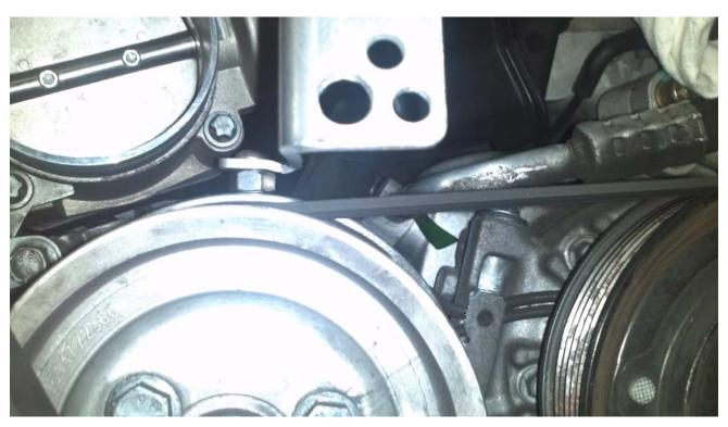
I used a rubber electrical box grommet as a standoff spacer and mounted the heat shield to the car body and bracket. I also used some rubber I had to make a gasket/cushion to prevent the intake pipe from rubbing on the heat-shield although there is actually clearance between them.
