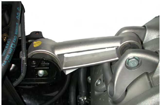
An additional torque strut on the cylinder head absorbs the high torque produced by the V8 engines.
