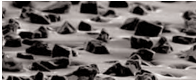
Illustration above shows the surface of the friction disk viewed under a microscope.
