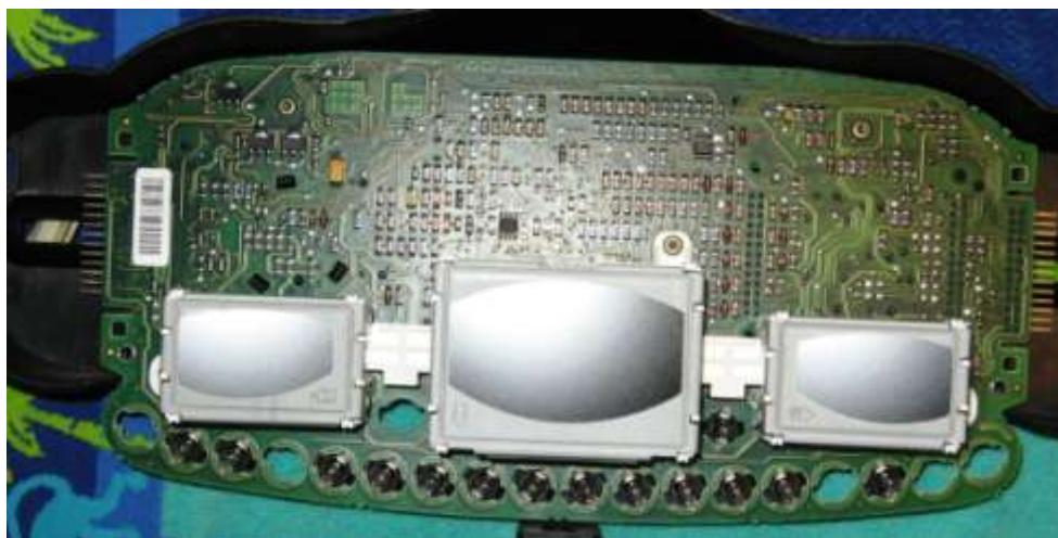
cluster. You can see the chip in this picture. It is the small, almost square, black chip that is above the center lcd and slightly to the right of the upper left corner of the lcd.
