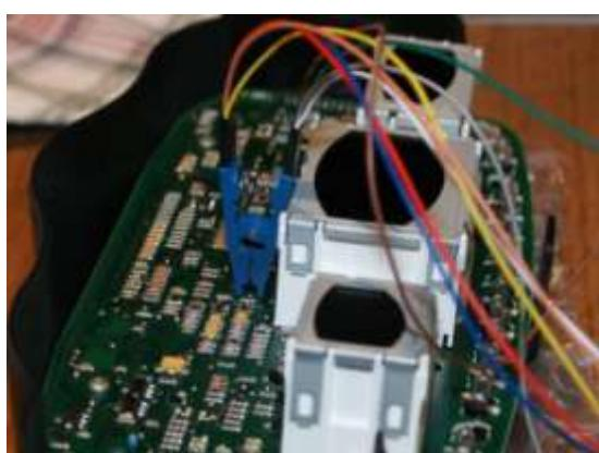
Here's a view of the SOIC clip attached to the circuit board. Once the clip is on the chip and the cable plugged in to the programmer you should select the chip type in the programmer software as a 93c56. Note that there are several choices for 93c56 chips in the
