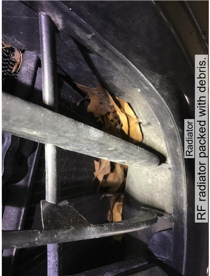
LF radiator packed with debris. Note that a coolant smell was detected from the front
