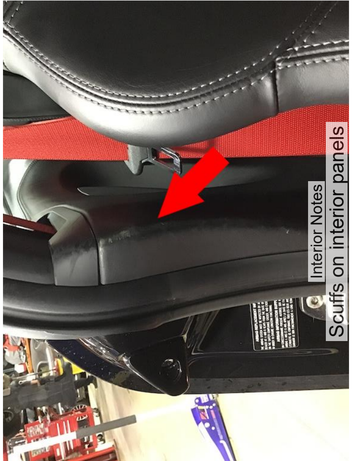
Interior Notes Scuffs in interior panels
