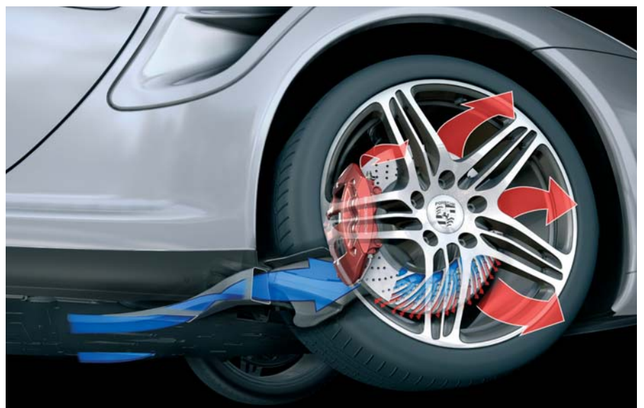
Fig. 34: Active venting of rear-axle brakes
