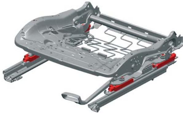
Fig. 54: Seat rail with weight detectors
