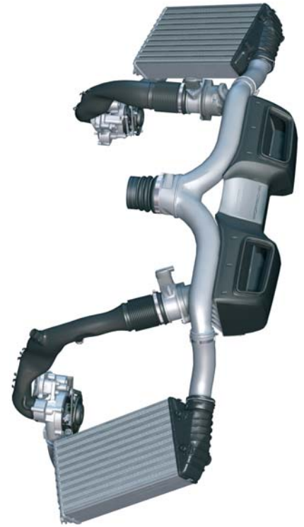
Fig.25: Air cleaner, air ducts, intercoolers
