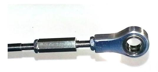
Adjustment will move shift lever position. Be sure to have lever in desired position before securing (tightened).
