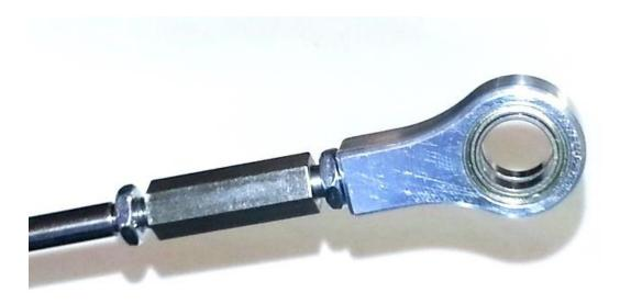
The ball bearing rod end is fully adjustable and attaches to the left side of the shifter (not tightened).
