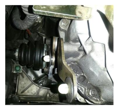
This transmission picture view indicates the yellow plastic inserts applied on the transmission cable posts before rod end fitment.
