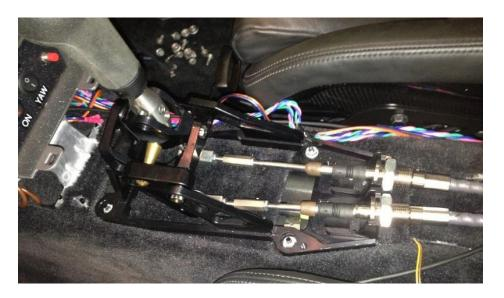
This picture indicates the <u>CORRECT</u> way to run the cables OVER the bracket.
