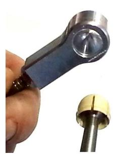
When installing the cables components make sure to apply the plastic caps to all ball end mounts.
