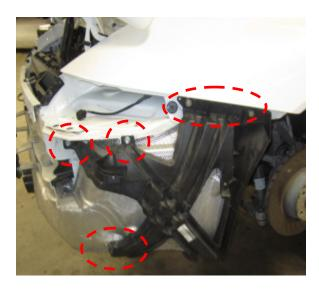
9. Now carefully remove frame-work on both sides. Next remove 5mph bumper (and its thin lower heatshield that is permanently attached) by removing two large vertical bolts with a 16mm
