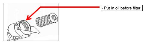
Step 13: Tighten oil filter housing to 25 N-m
