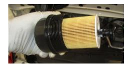
**Step 8**: Clean oil housing thoroughly and replace the two O-rings. Coat O-ring with small amount of oil **Step 9**: Suck out any oil that was left in the aluminum filter housing on the engine.
