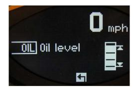
The above oil level reading is a maximum value, if the bar above the top arrow is illuminated, some oil should be drained from the system and the level checking procedure repeated.
