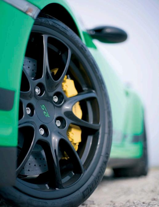
PCCB (left) is optional on both cars and adds to the weightsaving programme. RS is 20kg lighter than regular GT3 thanks to perspex rear window and carbon-fibre engine cover
