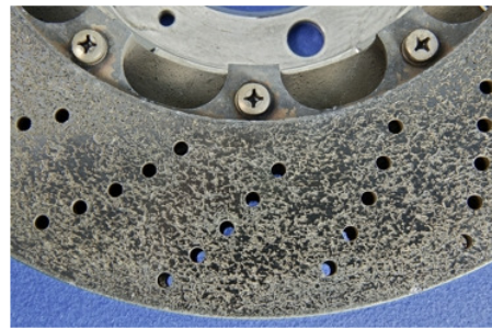
PCCB surface roughness (Sr) = 72 micrometre (view 1)
