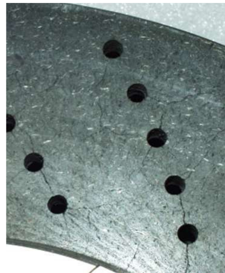
Stress-relief microstructure in PCCB brake disc friction surfaces
