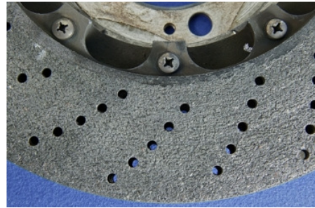
PCCB surface roughness (Sr) = 108 micrometre (view 1)
