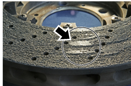
PCCB surface roughness (Sr) = 108 micrometre
