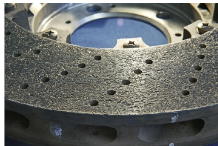
PCCB surface roughness (Sr) = 72 micrometre (view 2)
