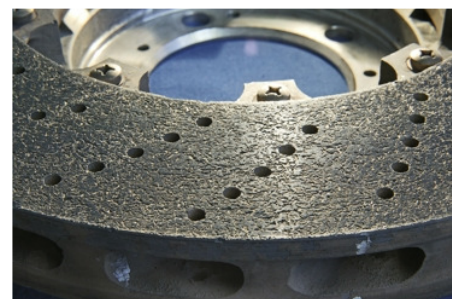
Surface roughness of PCCB brake disc
