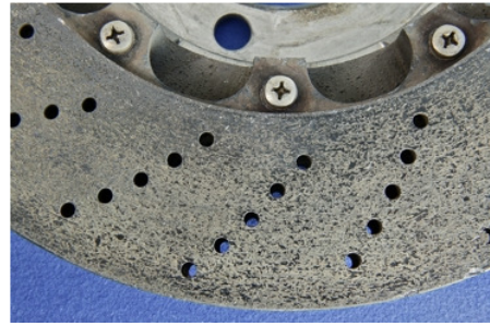
PCCB surface roughness (Sr) = 56 micrometre (view 1)
