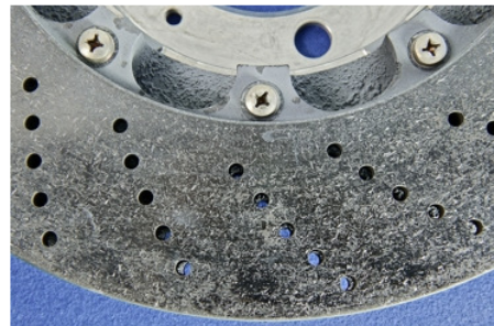
PCCB surface roughness (Sr) = 6 micrometre (view 1)
