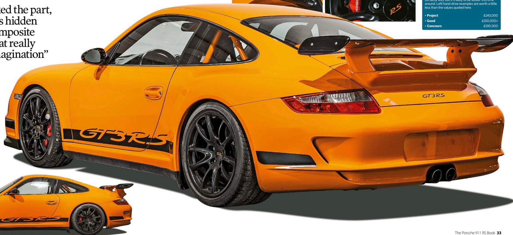
The 997.1 GT3 RS standard specification included 350mm steel discs clamped by six piston monoblock aluminium calipers at the front, and four piston items at the rear. Customary front bonnet vents and carbon rear wing aids downforce
