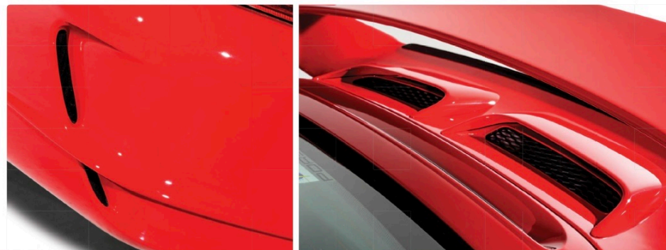
A variety of gills in the rear of the GT3 helped dissipate heat from the high-revving, dry-sump Mezger engine
