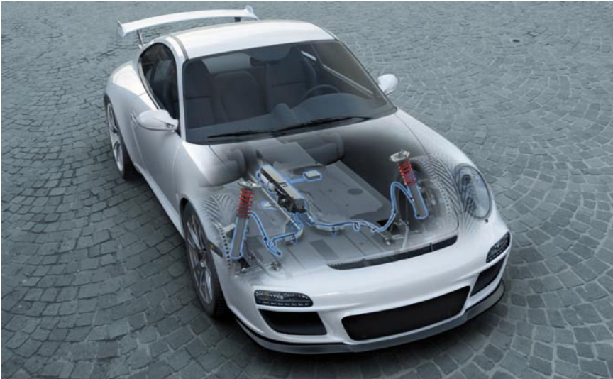
3 Lift system at the front axle of the GT3
