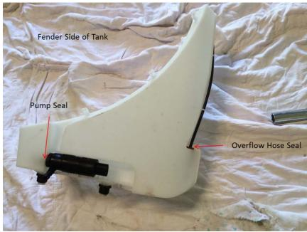
Installation of the tank is the reverse of removal. You will have to apply pressure and wiggle the tank to get the round peg grommets to fully seat in the fender sockets. Note the routing of the headlamp washer hose after you reattach it to the pump as below.
