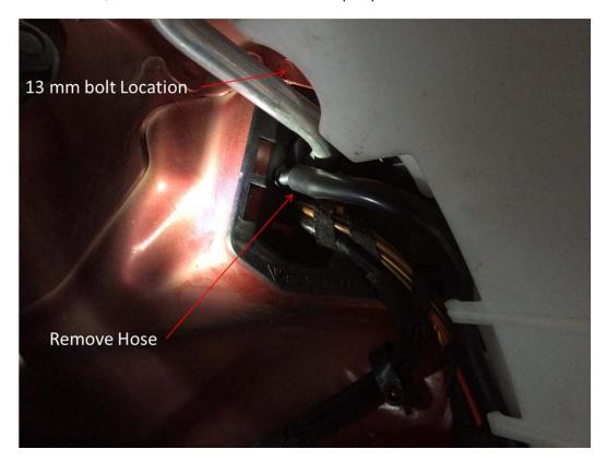
Once the bolt is out and the hose disconnected, grab the tanks and wiggle it out of the fender. It's being retained at this point with two round pegs with rubber grommets at the back of the tank, so it will take some nudging to get them to release.
