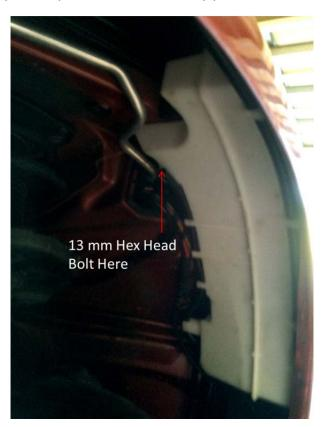
The tank is secured to the fender with one bolt requiring a 13 mm hex head socket. This bolt is located at the top of the tank at the approximate location shown above, also the location below with the tank removed. Its 1.5" long, so many turns of the socket wrench to remove.
