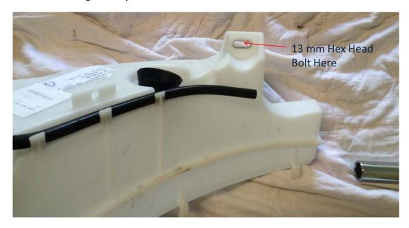
Before removing the tank, disconnect the windshield washer pump hose from the interface block below. Since this connector is plastic, use caution in removal to prevent breaking it. As far as the headlight washer's hose, I found it easier to remove from the pump once the tank was out.
