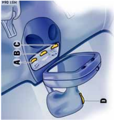
A, C - Switch for reading light on driver/passenger side B - Switch for interior light and footwell lights D - Orientation light
