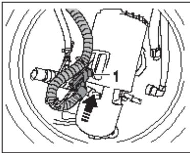
*Connecting sucking jet pumps to pump*
