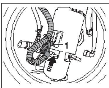
*Connecting sucking jet pumps to pump*
