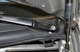
After removing the nut securing the wiper arms, simply pull the arms towards you. The plastic cowl is held in place at three places on top and two places just under the trunk lid behind the battery.
