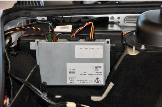
Next is running the cable harness up between the CD changer and the amp, directly behind the carpeted walls.
