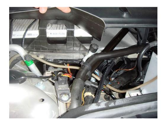
Reinstall cowl, run and secure excess antenna wire with cable ties. Run antenna lead through grommet into trunk.
