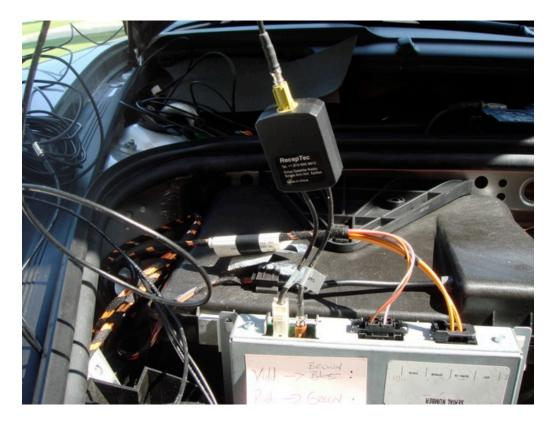
Connect the antenna lead to the antenna single to dual adapter and adapter dual leads to corresponding tuner leads. (Note in my case I had to remove plastic molded connector hosing from antenna adaptor.) Secure adaptor with double sided tape to side of tuner.
