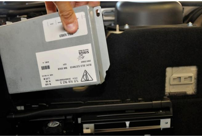
Next Step was to tap and connect power leads and fiber MOST connectors. As I already had a stock CD Changer, Nav and Bose system installed, using Porsche cable part number 955.044.900.65 it is the Harness for installs w/ CD Changer (provides MOST Fiber loop & Power adapter). Using this harness makings the install very easy. The cable has "Y" connectors for both power and fiber optic loop (MOST) connection.
