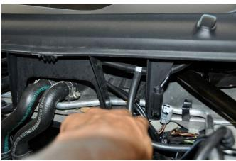
Next is mounting the satellite antenna to the underside of the cowl. Remove the cover secure with "push pins" (pry out with flat head screwdriver).
