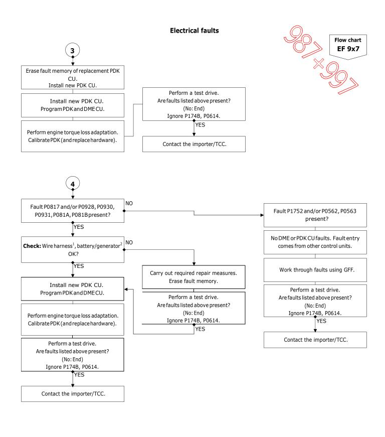
DME CU = DME control unit PDK CU = PDK control unit Electrohydraulic CU = Electrohydraulic control unit EPA = Electric pressure adjuster
