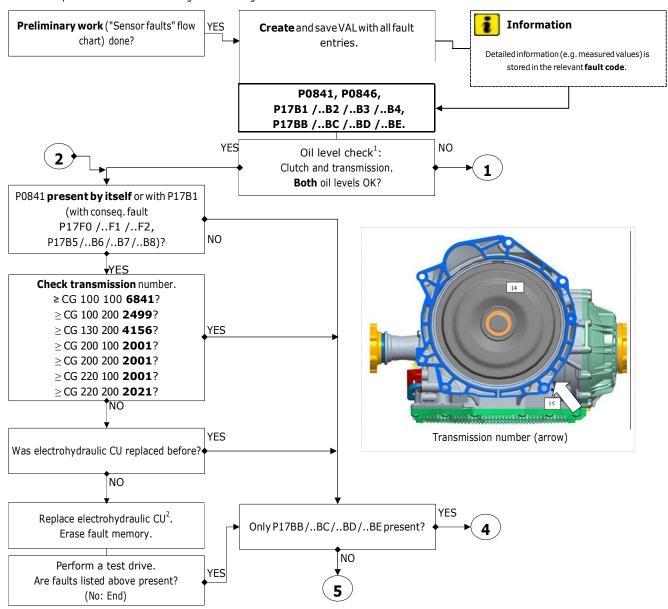
PDK CU = PDK control unit Electrohydraulic CU = Electrohydraulic control unit
