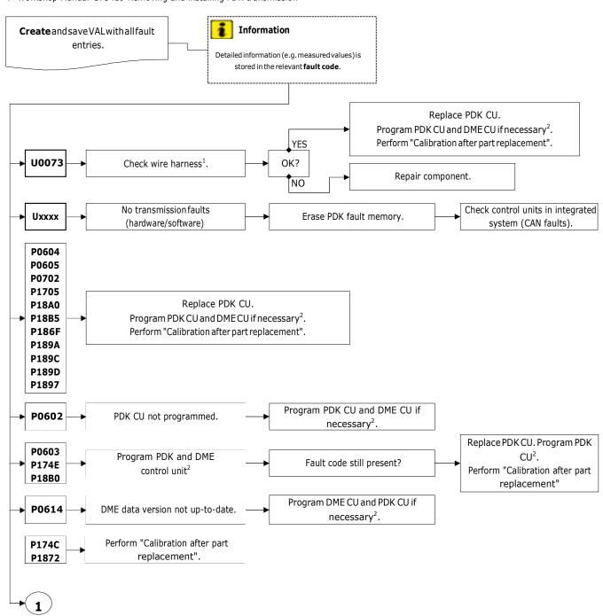
DME CU = DME control unit PDK CU = PDK control unit Electrohydraulic CU = Electrohydraulic GFF = Guided Fault Finding with PIWIS Tester 9718 PDK = Porsche Doppelkupplung control unit
