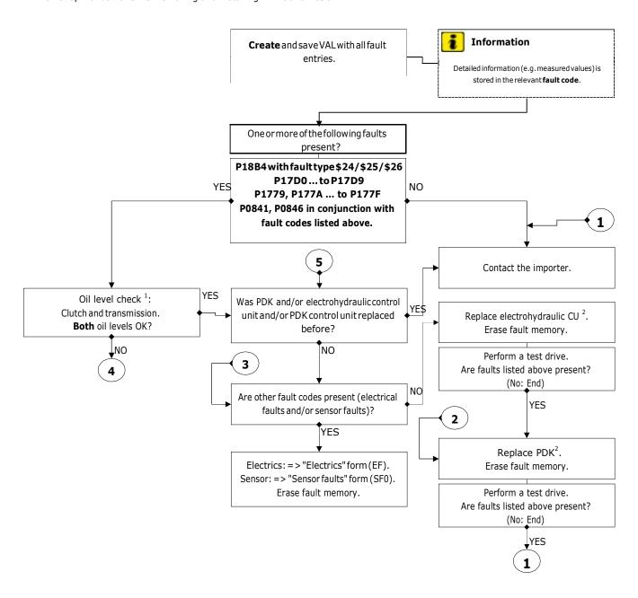
PDK CU = PDK control unit Electrohydraulic CU = Electrohydraulic control unit
