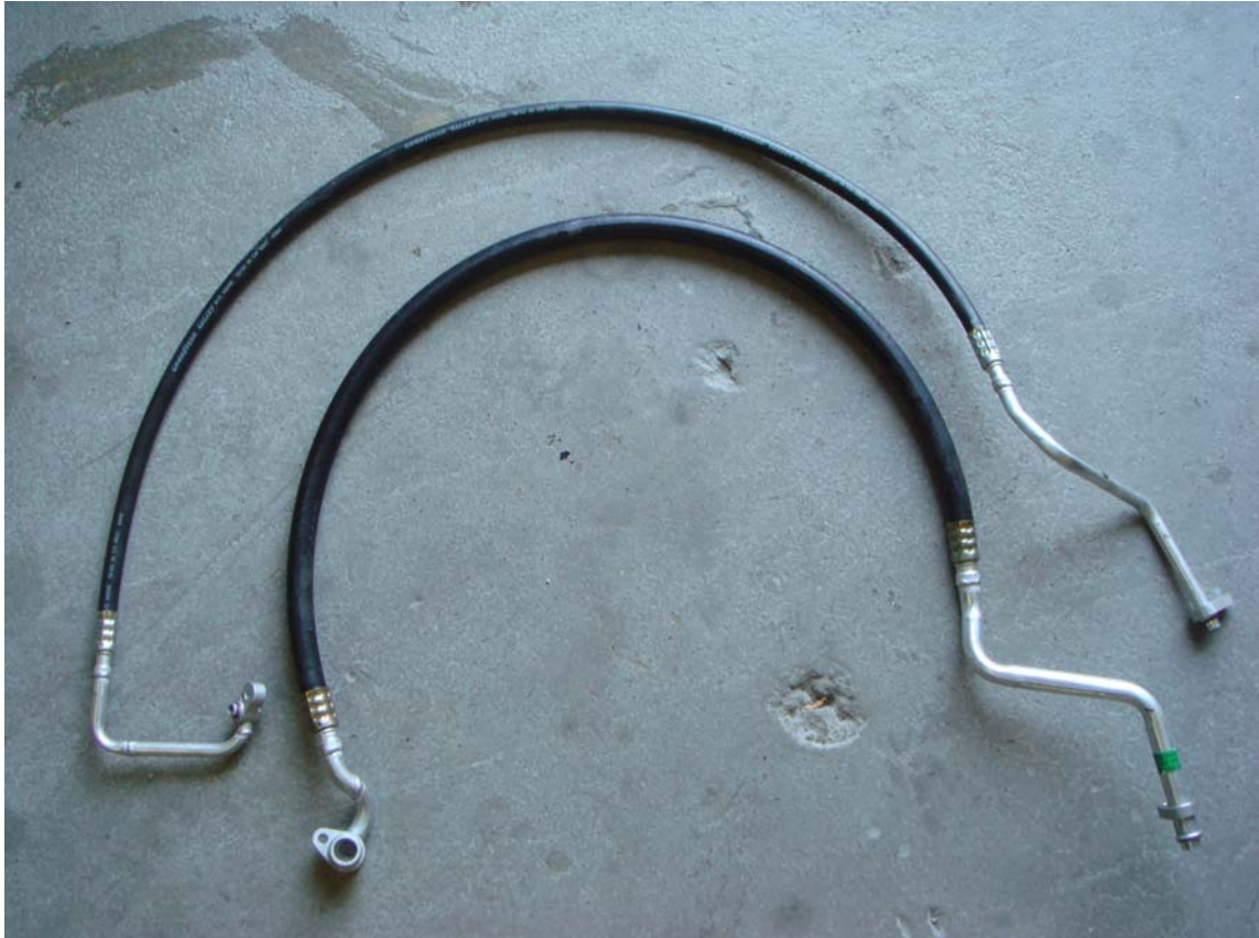
Figure 5.5 – Modified A/C Lines
