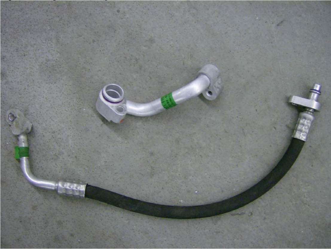
Figure 5.1 – Separate Compressor Fittings
