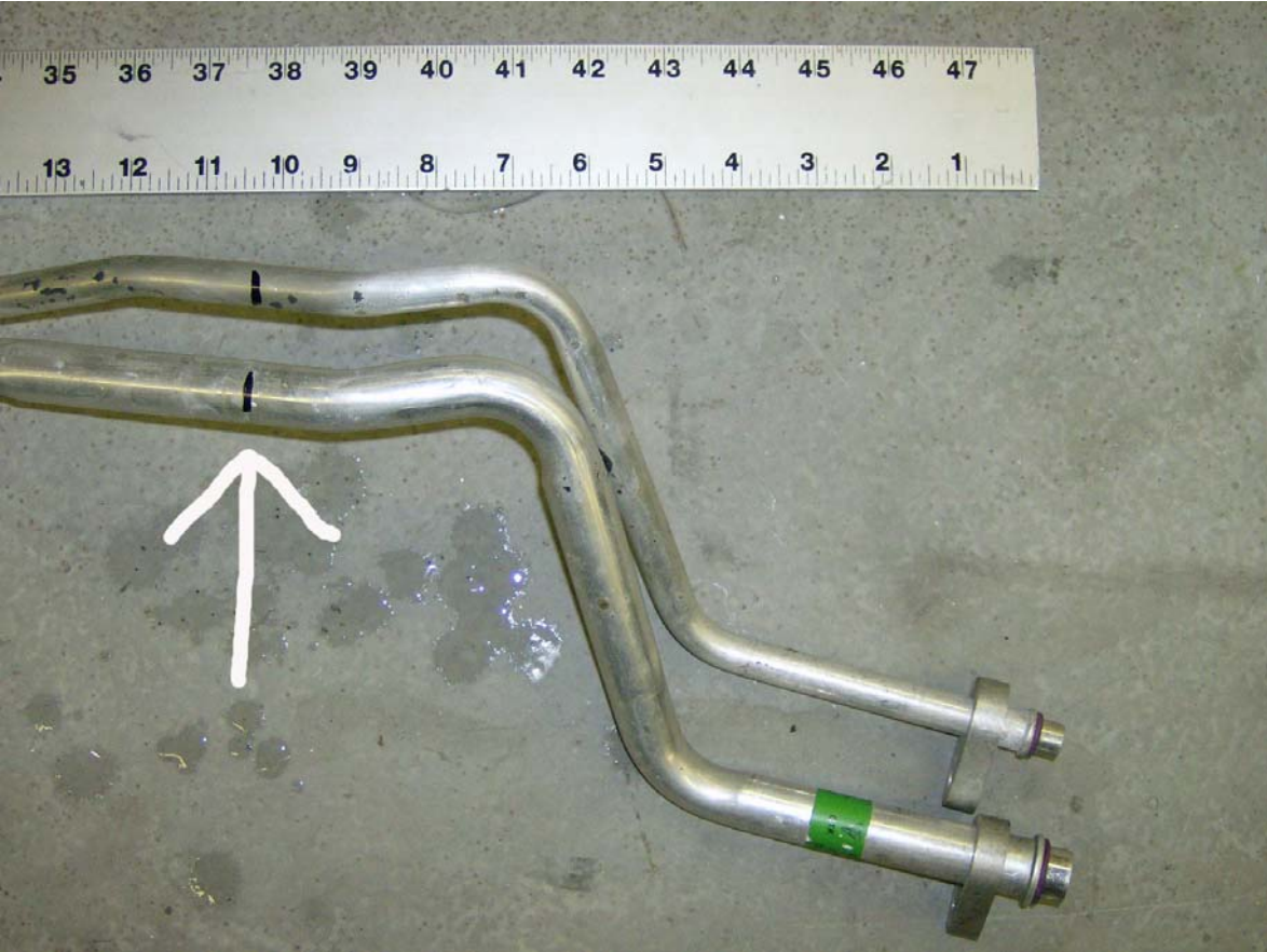
Figure 5.2 – Cut-off the End at the Arrow
