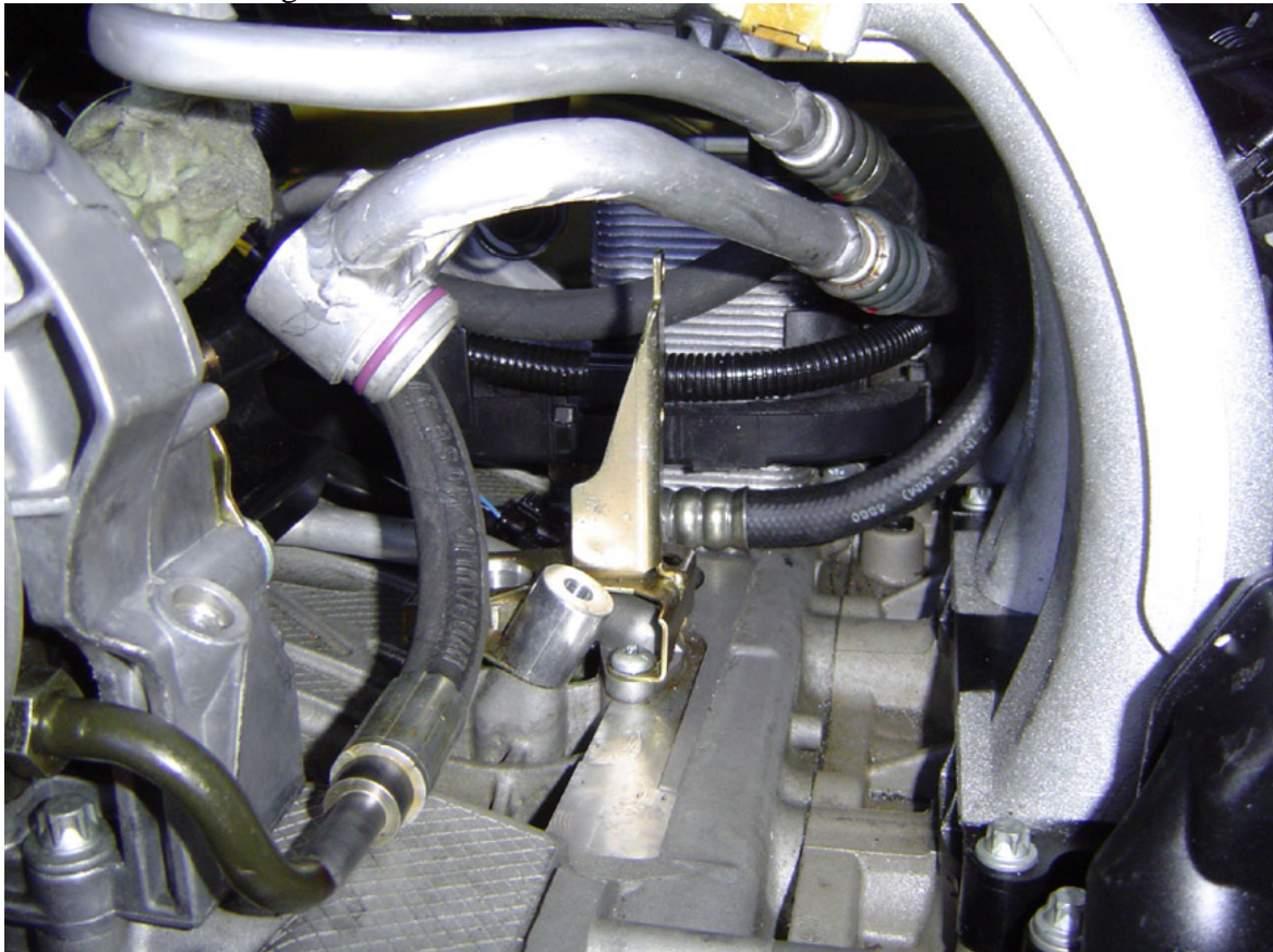
Figure 5.6 – A/C Lines Routing
