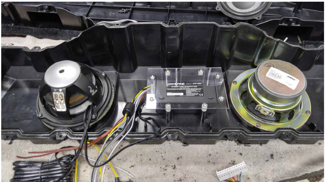
Comparison between the Focal sub on the left and the OEM Bose sub on the right - too bad noone can see the quality of the Focal unit since it's sealed up in a box.
