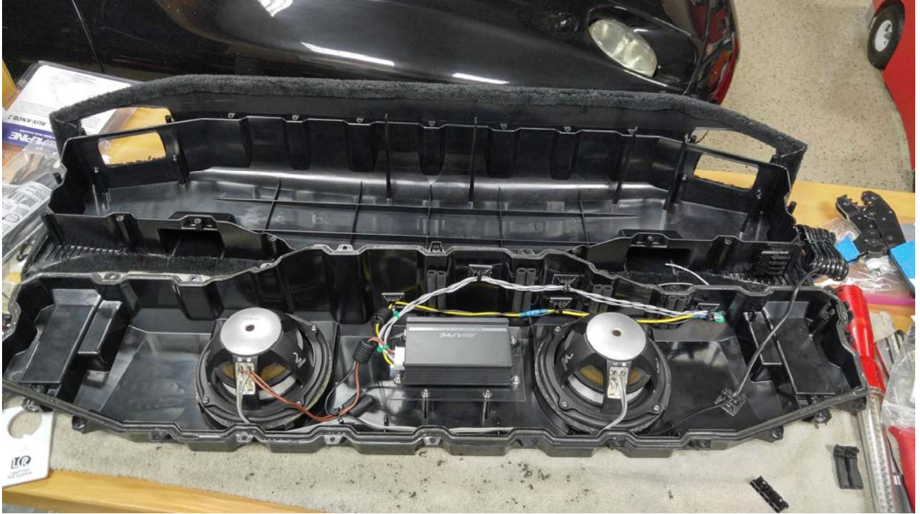
Completed and wired rear sub box.
