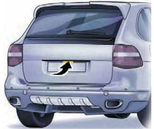
Option 1 – Press the release button on the rear lid.
