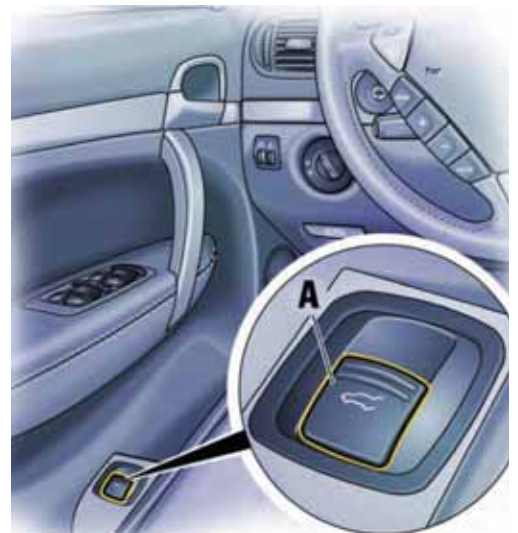
Option 3 – With the ignition switched on, pull the switch in the driver's door and hold it until the rear lid is fully open.
