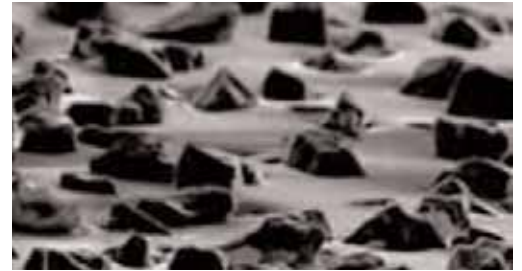
Illustration above shows the surface of the friction disk viewed under a microscope.
