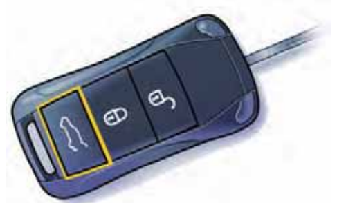
Option 2 – Press the button on the key for approx. 1 second.
