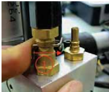
Removing the quick connectors.
