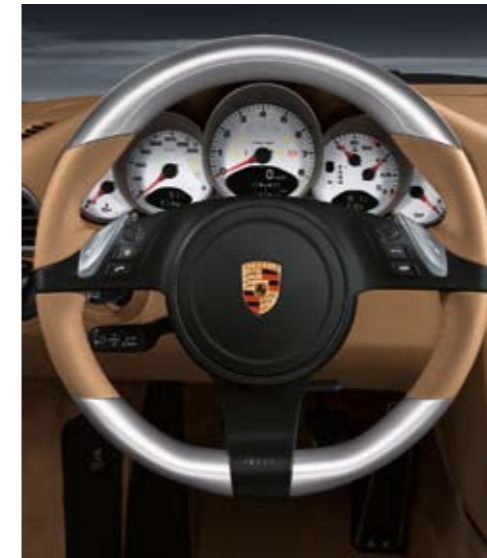
Three-spoke multifunction steering wheel in combination with PDK in Aluminium Look
