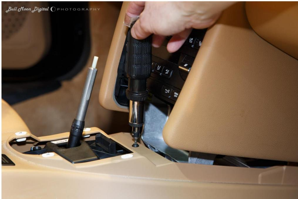
Step 9 – Use a T-20 Torx to remove a screw on each side that holds the center console to the car in the foot well area.
