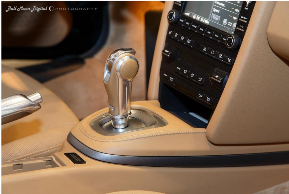
Step 2 – remove the shift knob. There is a collar at the bottom of the knob that turns counter-clockwise (as shown in the photo) to release it from the shaft. MACarbon suggests putting painters tape over it to increase the grip and make it easier to turn – I didn't need to do that this time. Once turned, pull up firmly but gradually – you don't want it to suddenly release and jerk you into the PCM or the rear view mirror.
