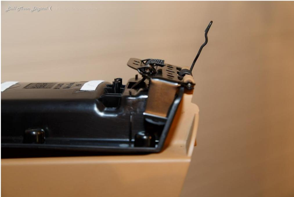
Step 20 – Lift up the hinge and the catch strap comes out of the lid – set the lid aside.
