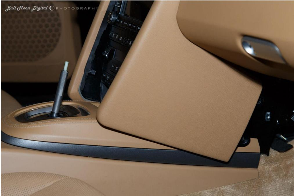
Step 5 – With the side panels loose, use a trim tool to gently pry up the console trim. There are clips at the rear, along the sides, and the front of the trim piece – pry straight up, not side to side!, and they will release. Take your time. Lift the shift trim up and out.
