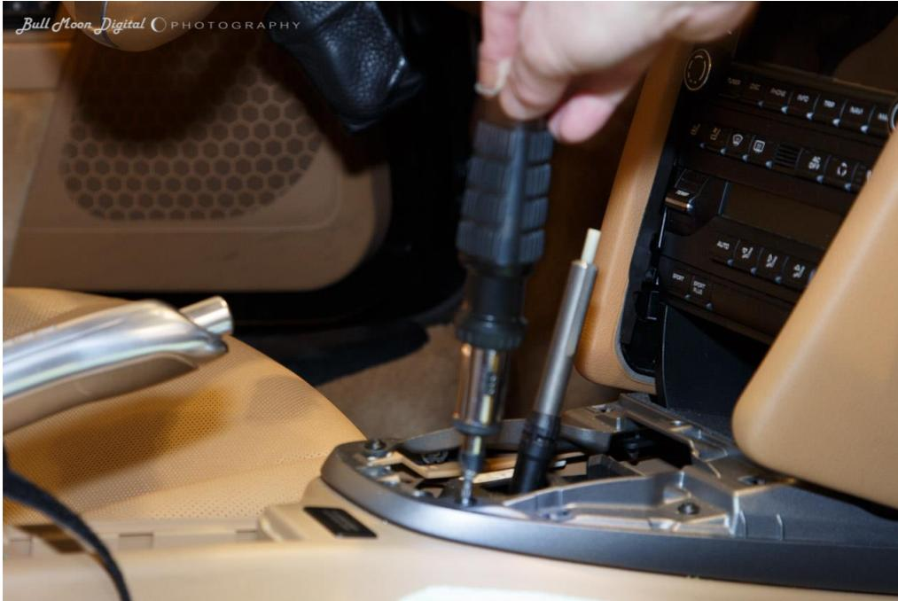
Step 7 – Using a T-20 Torx, remove a screw on each side of the storage bin. SLOWLY pull the storage bin out of the center stack; there is a tab at the top of it that clips in underneath the row of buttons above it – when I pulled mine out, the row of buttons came forward about ¼ inch and then I was able to disengage the tab and get it out – and push the row of buttons back into place.
