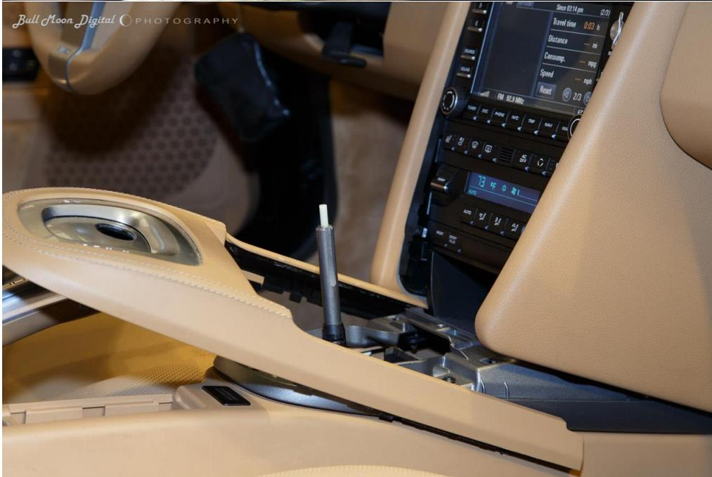
Now might be a good time to get the key out of the ignition to stop the chiming. I put the PDK knob back on loosely and put it in Park and removed the key. Then I carefully removed the knob again.
