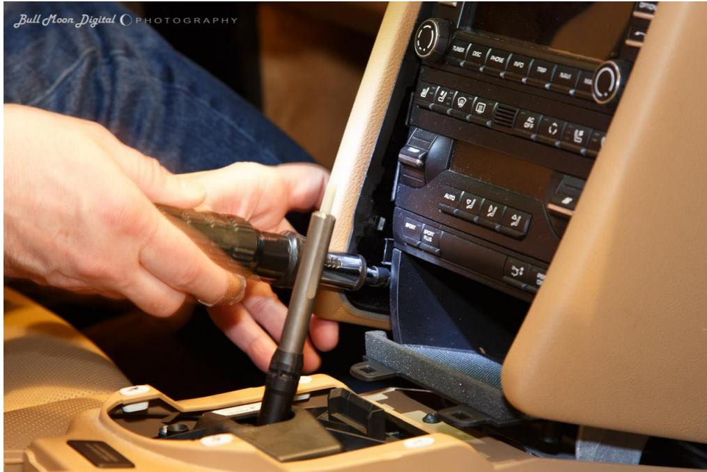
Step 8 – The removed bin allows access to a T-20 Torx screw holding the center console to the car. Remove that screw.
