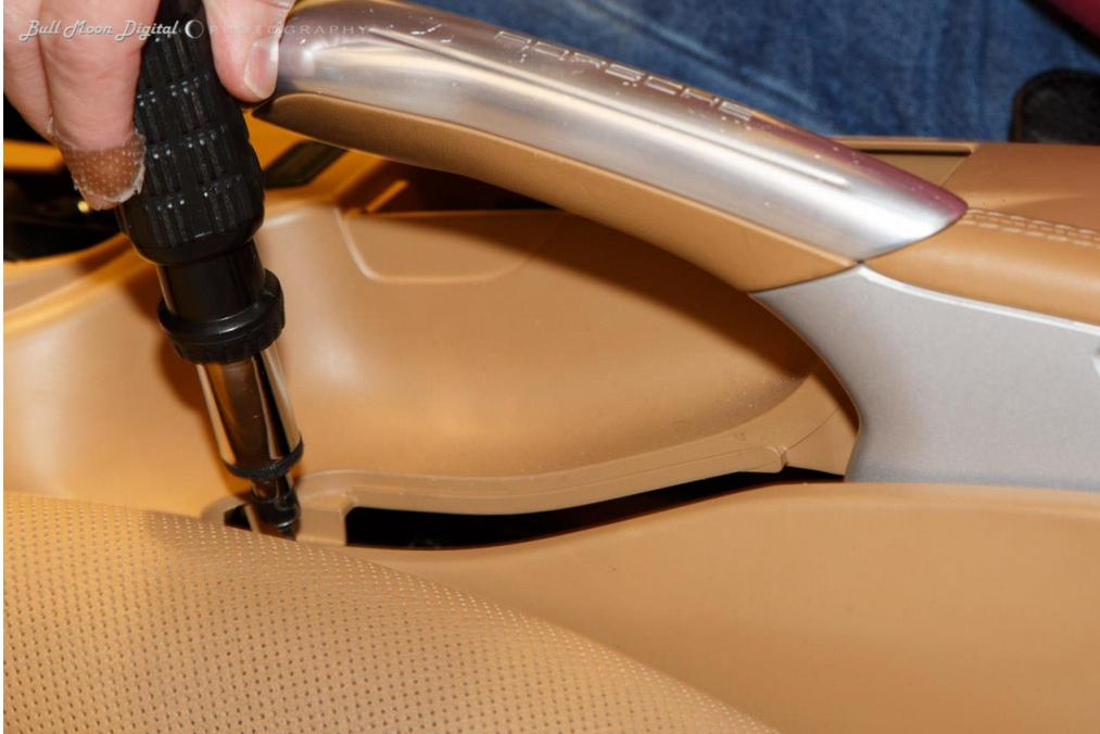
Step 15 – Back to the console stack where the front bin was removed and on the passenger foot well side, there is a plug that connects the center console wiring. There are release clips on each side where the wires come out that need to be pushed in slightly. They also need to be pressed in when replacing the plug later. Either reach under the console stack or around from the foot well and remove this plug.
