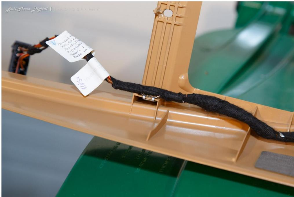
Step 25 – remove the Airbag indicator light – push it up out of the top of the center console – the metal clips on it barely hold it in.
