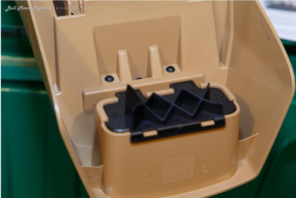
Step 18 – View from the back of the center console with rear bin removed and lid raised. This is how things should look when you put all the parts back together later. Now, let's take it apart so we can transfer the lid and spring hinge mechanism to the replacement center console.
