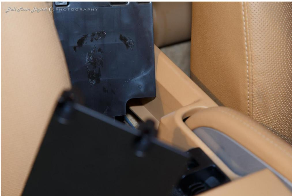
Step 13 – There are two cables and plugs connecting the iPod interface. As seen below, the plug on the left is rectangular and plugs straight down – there is a release clip on it and unhandily located behind it, but it is not that hard to release. The plug on the right in the photo connects a coax cable and plugs into the interface with a 90-degree connector. It also has a small release clip on it. This plug pulls out to the side rather than up.
