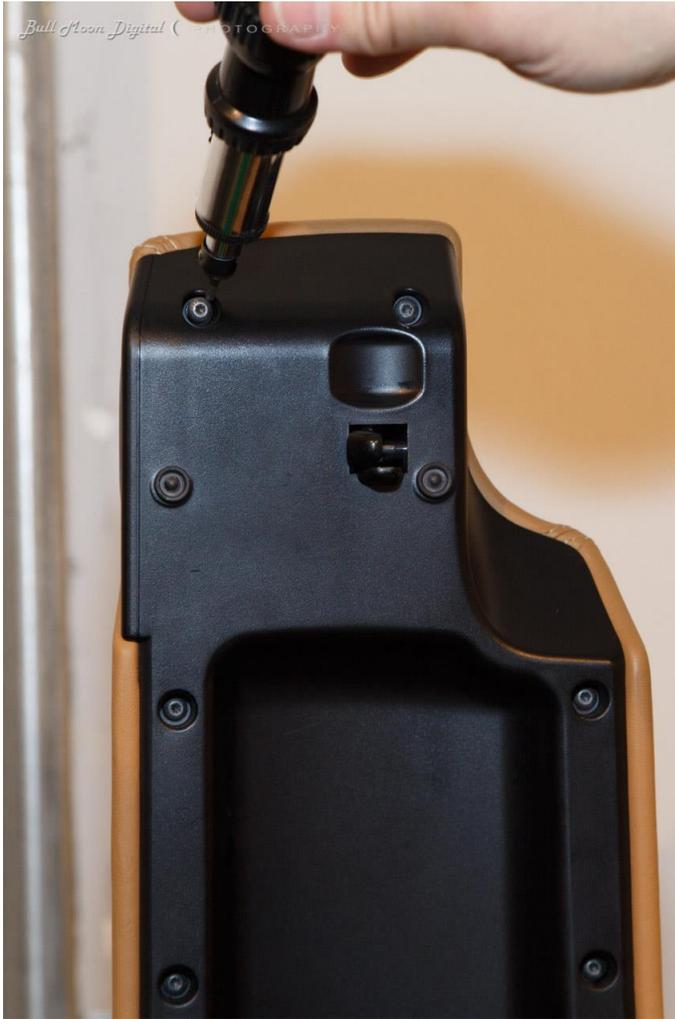
Step 17 – With the center console turned over, use a T-20 Torx to remove 2 screws that attach the rear storage bin to the center console. Lift the bin up to separate it from the console. This will give easier access to removing the center storage area lid. And you'll need all the advantages you can muster.
