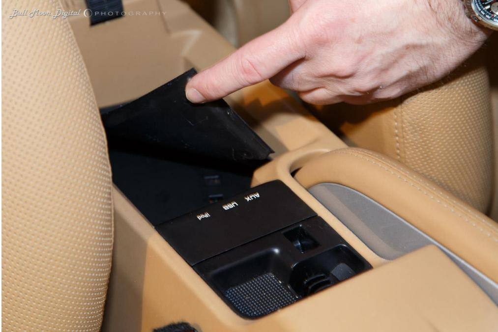
Step 11 – Use a T-20 Torx to remove the screws in the storage compartment. If the iPod interface is installed (as shown below), there will be 3 long screws visible, 4 screws if no iPod interface.
