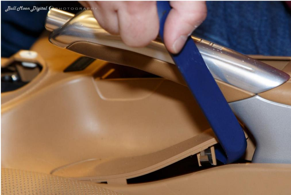
Remove the FINAL! T-20 Screw holding the Center Console in. Be careful not to drop it into the console when re-installing it!!!
