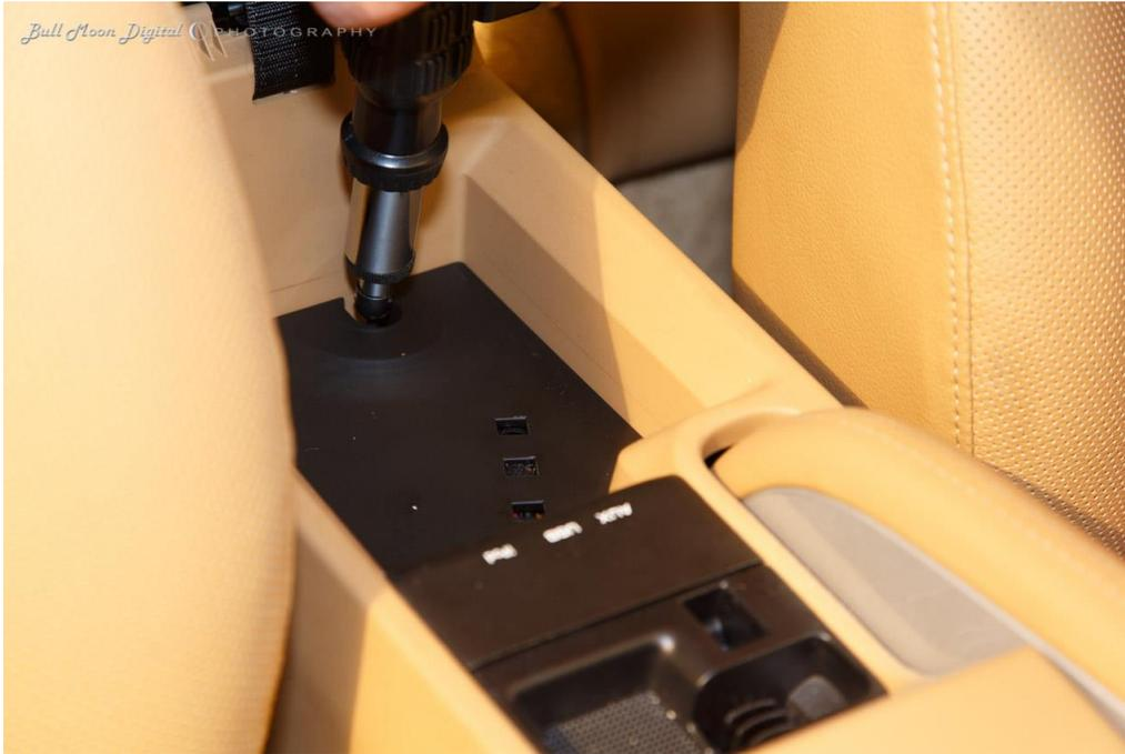
Step 12 – If installed, lift up the iPod adapter from the rear to remove it – this is not so easy to do and using a trim tool will help. Once out, the 4<sup>th</sup> short screw is visible – remove it and lift out the black “floor” plate.
