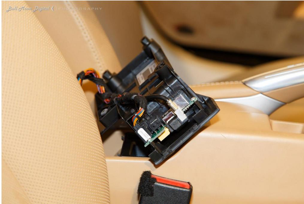
Both plugs shown disconnected. Remove the cables from the clips holding them to the iPod interface. The cables can be fed through the hole in the center console, later, when it is removed.
